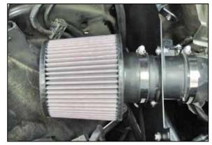
16. Install the K&N<sup>®</sup> air filter onto the mass air sensor and secure with the provided hose clamp.
