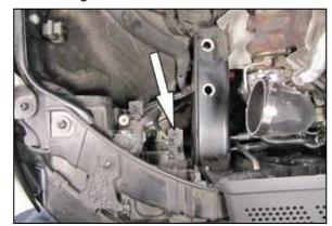
14. Remove the headlight mounting bolt shown.
