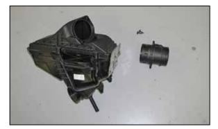
7. Remove the two screws securing the mass air sensor into the air filter housing and then remove the mass air sensor assembly from the air filter housing.
