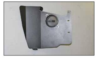
8. Install the mass air sensor assembly onto the heat shield as shown using the provided hardware.
