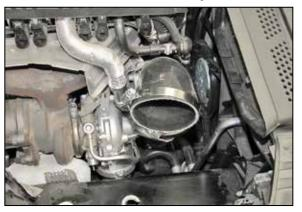
6. Install the provided turbo inlet hose (08490) onto the turbo and secure with the provided hose clamp. NOTE: Do not completely tighten at this time.
