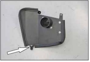
13. Install the insert nut onto the heat shield with the mounting bolt as shown.
