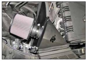
18. Install the K&N<sup>®</sup> fresh air intake duct and secure with the provided hardware.
