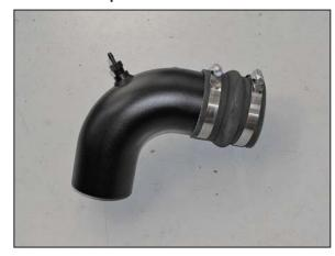
19. Install the remaining coupling hump hose (08696) onto primary  $K\&N^{\otimes}$  intake tube and secure with the provided hose clamp.
