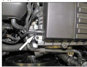
6. Disconnect the vacuum line from the air filter housing.
