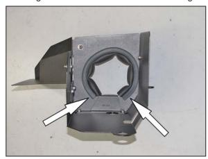
12. Install the 12.5" section into the heat shield as shown.
