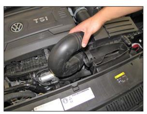
3. Release the fresh air intake tube from the tabs in the lower air filter housing and fresh air intake scoop and then remove the tube from the vehicle.
