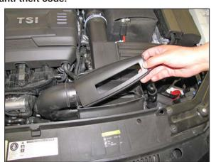
2. Release the fresh air intake scoop lid from the retaining tabs and then remove the lid from the fresh air intake scoop.
