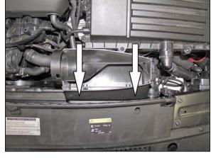
4. Remove the two screws securing the fresh air intake scoop to the core support and then remove the scoop from the vehicle.
