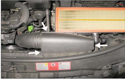
7. Release the three retaining clips securing fresh air intake lid and then remove the lid from the vehicle.
