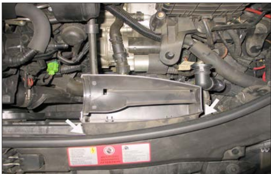
11. Remove the two screws which secure the fresh air inlet duct to the core support and then remove the duct from the vehicle.
