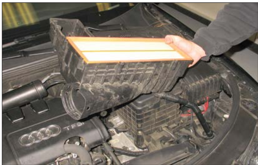
10. Lift the air box up to dislodge it from the mounting grommets and then remove it from the vehicle.
