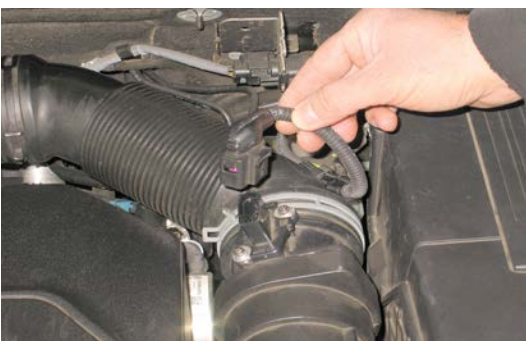
2. Disconnect the mass air sensor electrical connection.
