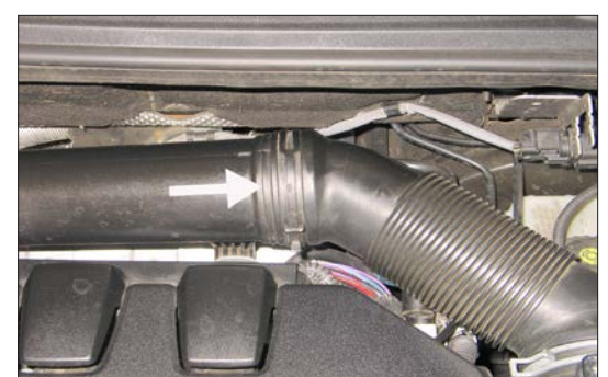
5. Release the spring clamp securing the factory intake hose to the factory intake tube and then unhook the intake hose.
