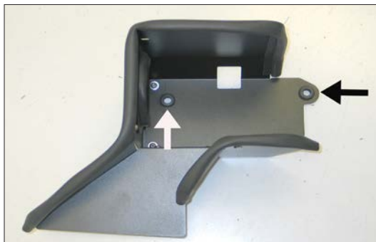
18. Install the two grommets into the base of the heat shield as shown.
