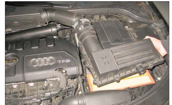
6. Remove the upper air box assembly from the vehicle as shown.
