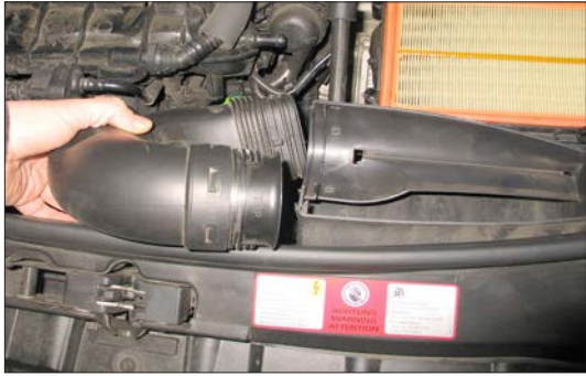
8. Disengage the fresh air intake duct from the lower air box and then remove the duct from the vehicle.
