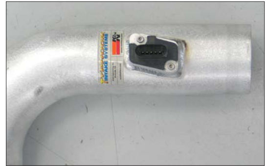
23. Install the mass air sensor into the K&N® secondary intake tube and secure with the provided hardware.
