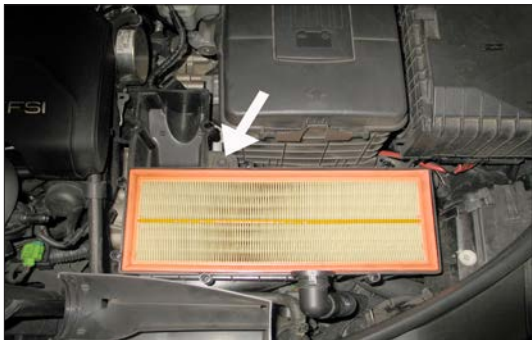
9. Loosen the bolt securing the lower air box to the vehicle.
