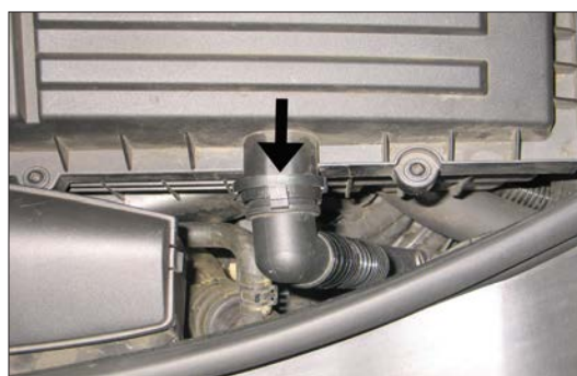
3. On vehicles equipped with an air injection system, release the air injection hose coupler from the upper air box half.
