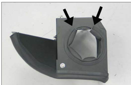
17. Install the 13" length of edge trim into the hole of the heat shield as shown.
