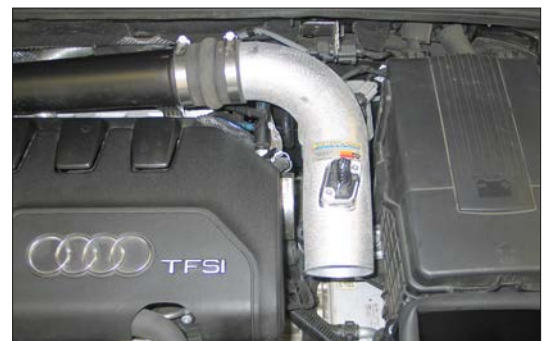
24. Install the K&N® secondary intake tube into the silicone hose at the factory intake tube and secure with the provided hose clamp.
