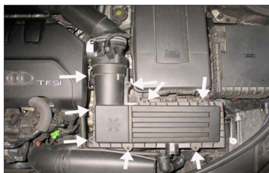
4. Loosen the eight screws securing the upper air box to the lower air box.
