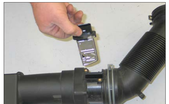
22. Remove the screws securing the mass air sensor and then remove the mass air sensor from the factory air box.
