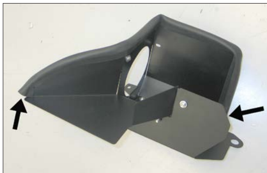
15. Install the 30" length of edge trim onto the heat shield assembly as shown.
