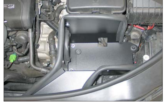
20. Set the heat shield into position on the air box mounting studs as shown and secure the mounting bracket with the provided hardware.
