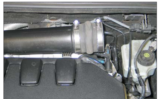
21. Install the provided silicone hump hose (08696) onto the factory intake tube and secure with the provided hose clamp.
