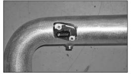
11. Install the mass air sensor into the K&N $^{\odot}$  intake tube with the provided hardware.
