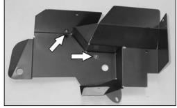
12. Install heat shield #07350 onto heat shield #07351 and secure with provided hardware.
