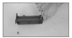
9. Using a small screw driver remove the two clip nuts from the lower fresh air duct as shown.
