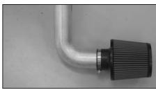
20. Install the K&N^ ${\rm \circledast}$  air filter onto the K&N  $^{\rm \circledast}\,$  intake tube and secure with the provided hose clamp
