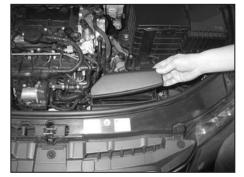
2. Disconnect the mass air sensor electrical connection and unhook the mass air sensor wiring from the engine cover.
