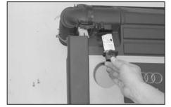
10. Remove the two screws that secure the mass air sensor to the stock air filter housing and then remove the mass air sensor as shown.
