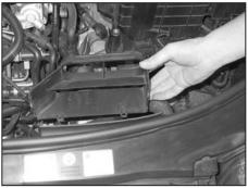
8. Unsnap and remove the lower fresh air duct as shown.
