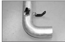
11a. Install the tube mounting bracket (070107) onto the K&N $^{\circ}$  intake tube and secure with the provided hardware.
