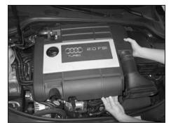
4. Pull up firmly on the air filter housing/engine cover assembly to release it from the mounting grommets.
