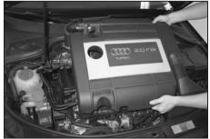
6. Remove the air filter housing/engine cover assembly from the vehicle.
