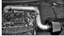
21. Install the K&N<sup>®</sup> intake tube into the silicone hose at the turbo inlet and align with the bracket installed during step 19. Secure the bracket attached to the intake tube (070107) to the airbox mounting location. Secure the intake tube with the provided hose clamp and hardware.
