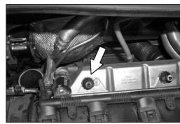
6a. Remove the airbox mounting stud shown
