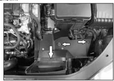
16. Install the heat shield assembly and fresh air duct into the vehicle so that the heat shield mounting grommets are snapped onto the mounting studs and the fresh air duct snaps into the fresh air supply tube, secure the duct and heat shield with the provided hardware. **NOTE: Be sure to snap the lower fresh air duct into the fresh air supply tube. The fresh air duct will bolt to the heat shield.**
