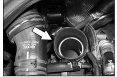
18. Install the provided silicone hose (084016) onto the turbo inlet and secure with the provided hose clamp.
