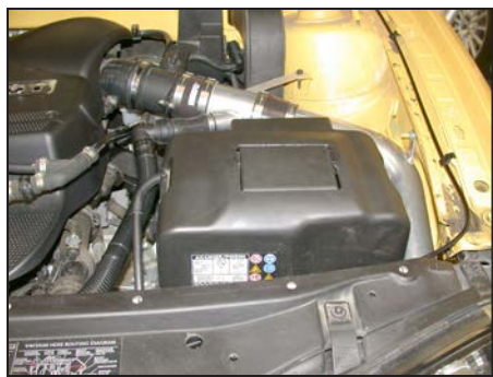
46. Reinstall the battery cover as shown.
