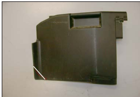
47. Trim the corner of the outer core support cover to provide clearance for the cold air tube as shown.
