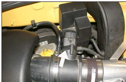
50. Reconnect the mass air sensor electrical connection as shown.
