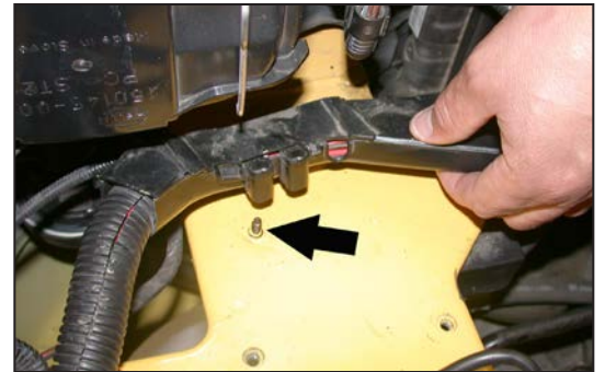
25. Remove the wire harness from the stud on the inner fender as shown.
