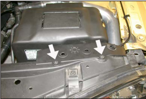
48. Reinstall the outer core support cover using the original screws as shown.
