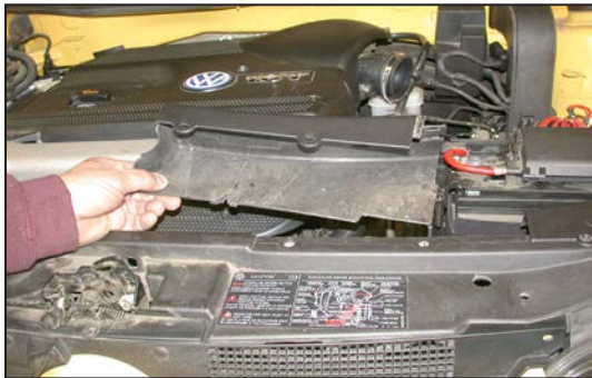
12. Remove the inner core support cover, which is secured by two screws.
