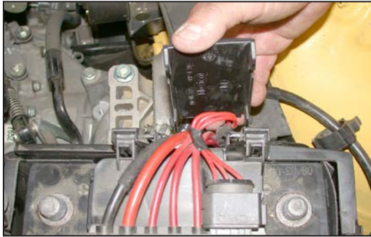
15. Slide the rear battery harness cover upwards and remove from the battery cover as shown.
