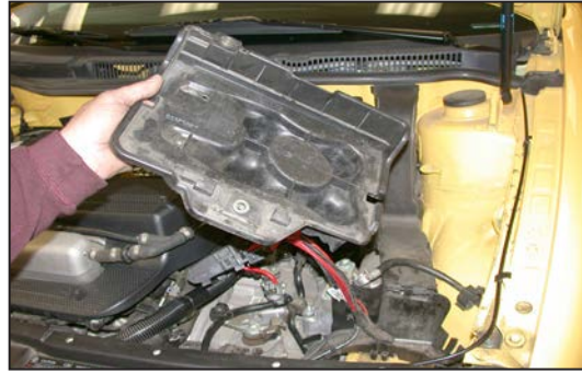
20. Remove the battery tray, which is secured by four bolts as shown.
