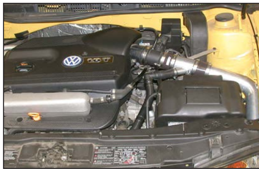
51. This K&N® high flow intake system has been designed to be used in two different configurations. In the case of inclement weather, the cold air tube can be removed and the air filter can be clamped onto the intake tube located in the engine compartment to avoid the possibility of ingesting water into the engine.
