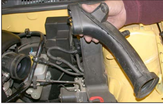
11. Remove the nut that secures the air inlet duct, then remove the air inlet duct as shown. NOTE: K&N Engineering, Inc., recommends that customers do not discard factory air intake.
