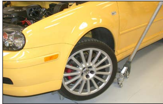
21. Lift the vehicle upwards and support it with jack stands as shown.
