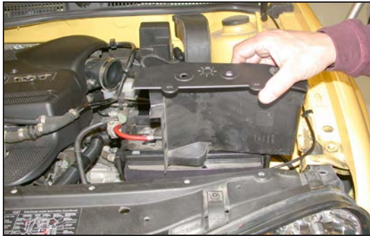
13. Remove the outer core support cover, which is secured by two screws.
