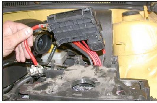
16. Slide the battery fuse/harness assembly backwards, then upwards as shown, and pull the battery fuse/harness assembly out of the way.
