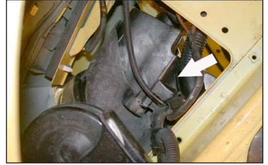
23. From underneath the vehicle remove the lower plastic rivet from the inner plastic headlight cover as shown.
