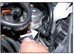
15. Depress the locking tab on the EVAP hose to release from the EVAP pump.
