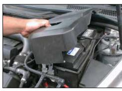
1. Turn the ignition OFF and disconnect the vehicle's negative battery cable by first removing the battery cover as shown.
