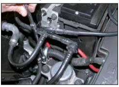
10. Loosen and remove the Delphi clamp bolt that secures the main wiring harness to the EVAP pump.
