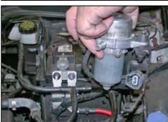
17. Loosen the two EVAP pump bracket mounting bolts and the main battery harness c-clamp bolt, then remove the EVAP pump from vehicle.
