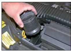
13. Twist and remove the accordion hose from the lower air inlet duct as shown.
