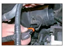
5. Disconnect the mass air sensor electrical connection as shown.
