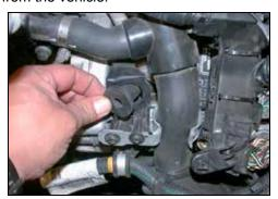
25. Install the provided threaded insert into the mounting hole from step 24.
