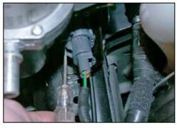
16. Disconnect the EVAP pump electrical connection by inserting a small flat blade screwdriver and depressing the locking clip while pulling the connector away from the harness.
