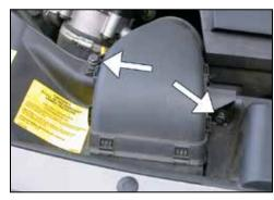
12. Loosen and remove the two screws that secure the upper air inlet duct, then remove from vehicle.
