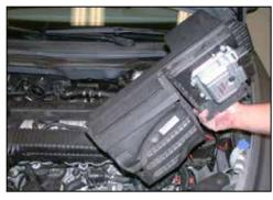
18. Pull firmly upwards to release the air box from the rubber mounting grommets, then carefully slide the air box towards the battery side of the vehicle; slowly remove from vehicle.
