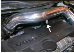
39. Secure the intake tube to the bracket with the provided hardware as shown.
