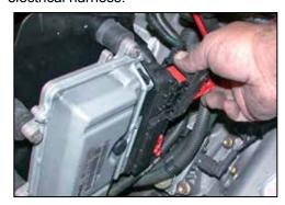
31. Re-connect the two electrical wiring harness to the ECM.
