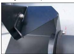
29. Secure the "L" bracket to the heat shield as shown but do not tighten completely at this time.
