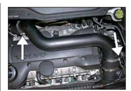
3. Loosen the two hose clamps that secure the stock intake tube.
