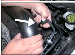
4. Lift slightly and remove the EVAP recirculation line. Remove the carbon filter vacuum hose by depressing the two locking tabs as shown, then remove the intake tube from vehicle.
