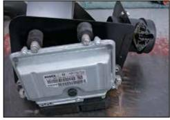
23. Mount the ECM onto the heat shield with the provided hardware as shown.
