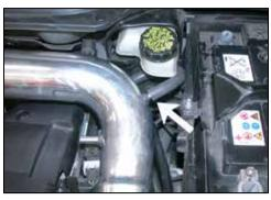
42. Connect the other end of the EVAP recirculation line hose to the vent tube on the intake tube as shown.
