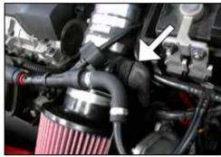
48. Reconnect the mass air sensor electrical connection.
