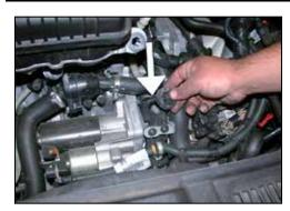
24. Remove the large air box mounting grommet from the vehicle.
