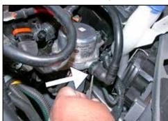
47. Reconnect the EVAP pump hose to the EVAP pump removed in step 15.
