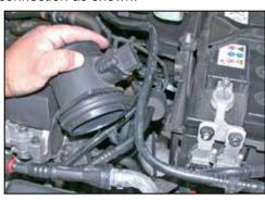
6. Using a Torx T25, remove the two bolts that secure the mass air sensor to the air box and remove from the vehicle.
