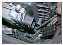
11. With a screwdriver, push down and out to release the slide clip that secures the harness bracket to the air box.
