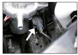
46. Reconnect the EVAP pump electrical connection detached in step 16.
