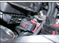
9. Depress the release tabs on the upper and lower electrical harness and disconnect from the ECM as shown.
