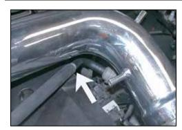
41. Insert the hose mender into the stock EVAP recirculation line as shown.
