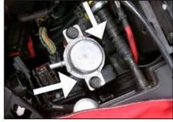
45. Reinstall the EVAP pump and secure with the two mounting bolts removed in step 17.
