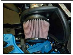
22. Install the K&N® air filter and secure with the hose clamp.
