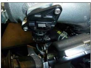
21. Reconnect the mass air sensor electrical connection.
