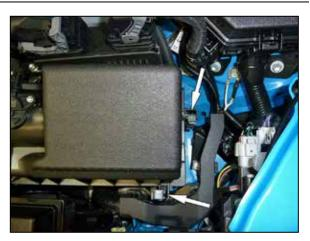
5. Release the upper air filter housing retaining clips, lift and remove the upper air filter housing and intake tube. Remove the factory air filter.
