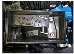
6. Remove the two bolts that secure the lower air filter housing and then remove the lower housing from the vehicle.
