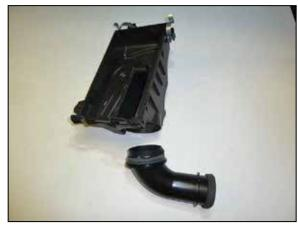
7. Separate the fresh air intake duct from the lower air filter housing.
