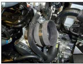
14. Install the provided coupler (08421) onto the throttle body and secure with the provided hose clamp.
