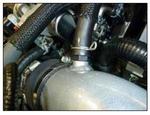
19. Connect the PCV hose to the fitting installed into the K&N<sup>®</sup> intake tube and secure with the factory spring clamp.
