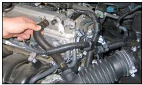
3. Disconnect the crank case vent hose from the valve cover port as shown.
