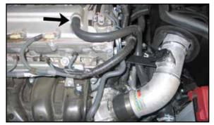
18. Install the crank case vent hose onto the valve cover port and then onto the K&N<sup>®</sup> intake tube. NOTE: Be sure to route the vent hose so that it is not kinked and then secure with the provided tie wrap. Some trimming of the vent hose may be necessary.
