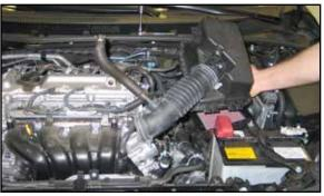
6. Unclip the upper air box retaining clips and then remove the upper air box and intake assembly.
