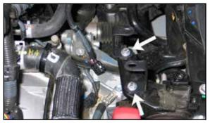
9. Install the two heat shield mounting brackets (070052) onto the air box mounting bracket as shown.
