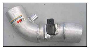
15. Install the mass air sensor into the K&N<sup>®</sup> intake tube and secure with the provided hardware.
