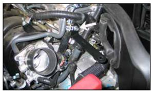
16. Install the tube mounting bracket (070110) onto the engine using the bolt removed during step #8.
