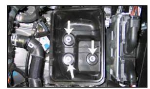
7. Remove the three lower air box retaining bolts. Then unclip the wiring harness from the rear of the air box and remove the lower air box housing from the vehicle.
