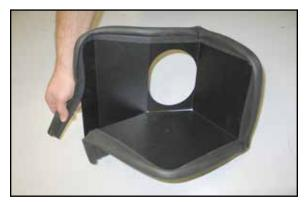
10. Install the provided long edge trim onto the heat shield as shown.
