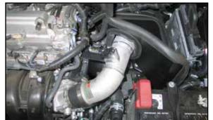
17. Install the K&N<sup>®</sup> intake tube into the silicone hose at the throttle body and align with the bracket installed in the previous step. Secure the intake tube with the provided hose clamp and hardware.
