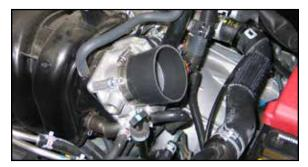
13. Install the provided silicone hose (084016) onto the throttle body and secure with the provided hose clamp.
