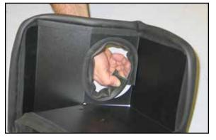
11. Install the provided short edge trim into the heat shield as shown.
