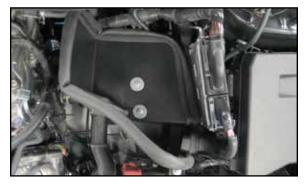
12. Install the heat shield assembly onto the mounting brackets installed in step #9 using the provided hardware.
