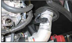
19. Route the mass air electrical harness through the heat shield as shown and then reconnect the mass air sensor electrical connection.
