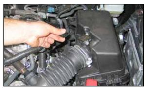
4. Disconnect the mass air sensor electrical connection. Then unhook the mass air sensor wiring harness from the upper air box.
