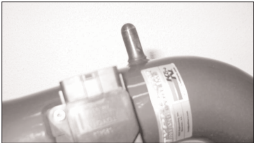
17. Fit the rubber cap plug over the vent of the Typhoon intake tube as shown.
