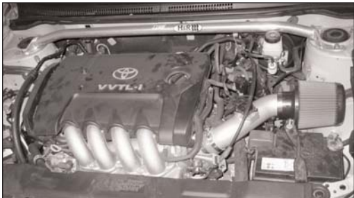
26. Re-connect the negative battery cable and double check that everything is tight and properly positioned before starting the vehicle.
