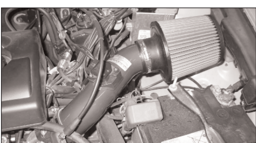
23. Adjust the filter assembly for clearance, then, firmly tighten all hose clamps and hardware connections!
