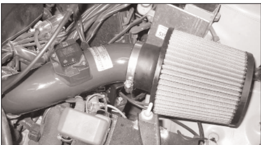
22. Install the Air Filter onto the Typhoon tube and secure with the provided hose clamp as shown.
