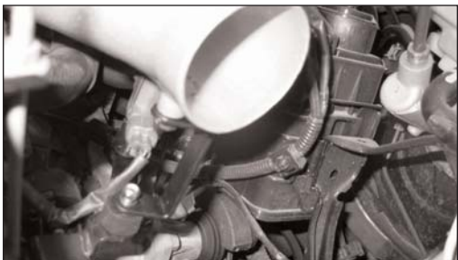
20. Align the tube with the "C" bracket and secure with the M6 bolt and wave washer supplied. Don't fully tighten yet!
