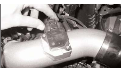
24. Re-connect the MAS electrical connection as shown.
