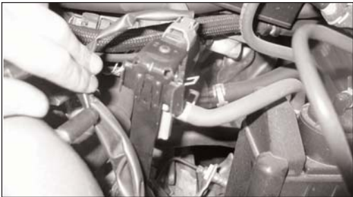
21. Slide the PWM vacuum switching valve onto the "L" bracket as shown.
