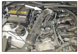
4. Loosen the two hose clamps securing the factory intake tube and then remove the factory intake hose from the vehicle.
