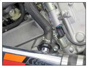
11. Install the crank case vent hose onto the fitting installed into the K&N® intake tube.
