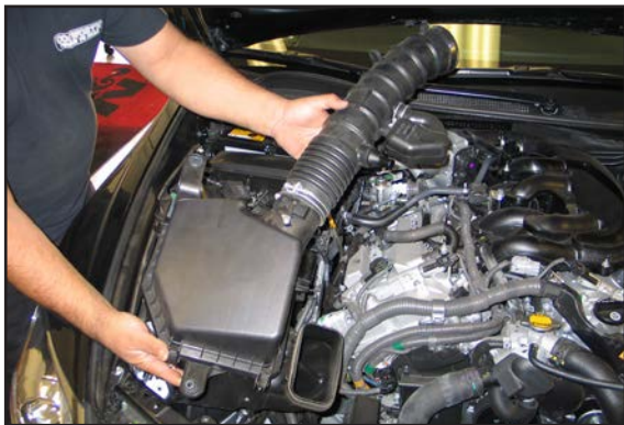
12. Remove the complete intake assembly. NOTE: Unhook the vacuum lines clipped onto the intake tube. NOTE: K&N® recommends that customers do not discard factory air intake.
