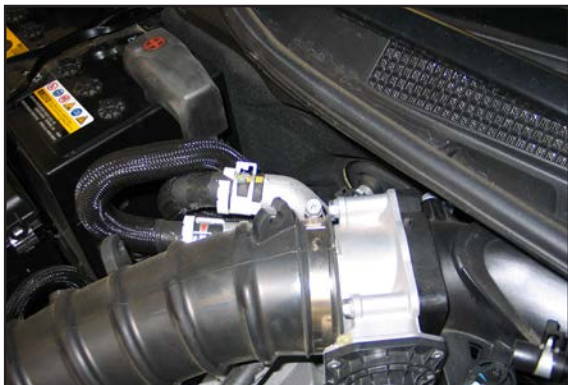
11. Loosen the hose clamp that secures the stock intake tube to the throttle body.
