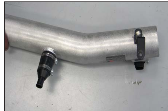
26. Install the "Z" (070992) onto the K&N® intake tube as shown. NOTE: the twist side of the bracket should be bolted to the tube.
