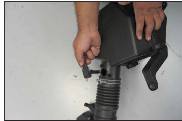
22. Remove the screws that secure the mass air sensor into the stock air filter housing and then remove the mass air sensor.
