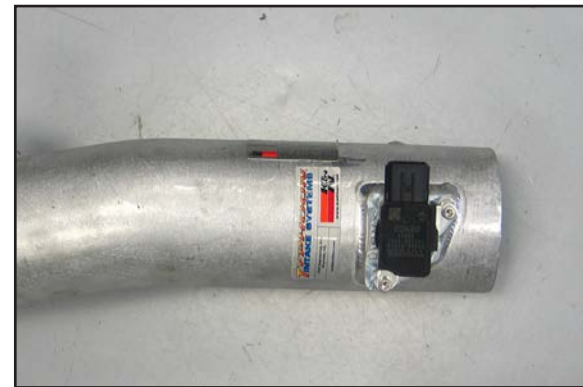
23. Install the mass air sensor into the K&N® intake tube with provided bolts.
