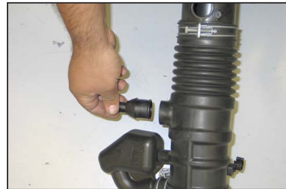
24. Remove the crank case vent chamber from the stock intake tube as shown.
