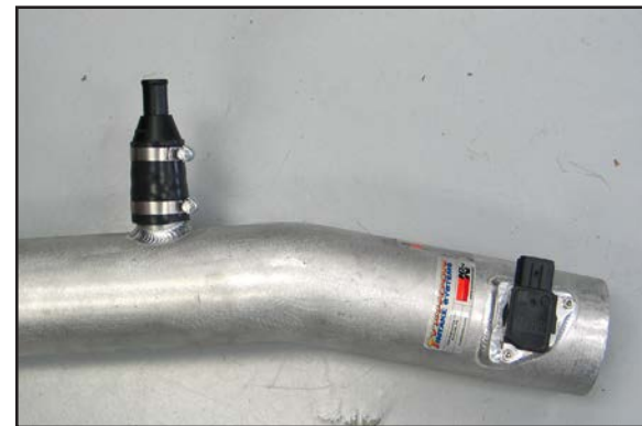
25. Install the silicone hose onto the K&N® intake tube crank case vent as shown and secure with the hose clamp, then install the factory crank case vent chamber into the silicone hose and secure with the hose clamp as shown.
