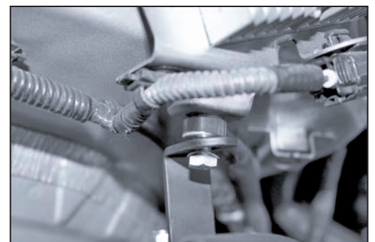
24. Line up Z bracket with the ground mounting bolt from step 23. With provided spacer, washers and bolt secure bracket as shown, make sure to reconnect the ground so that it is underneath the aluminum spacer.
