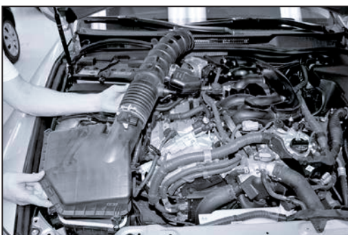
14. Remove the upper air box along with the factory intake tube as shown.
