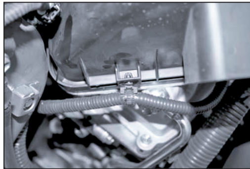
17. Rotate the air box 180° to access the MAF sensor wire harness tie down clip and release it with pliers.
