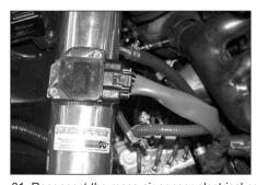
31. Reconnect the mass air sensor electrical connection as shown.
