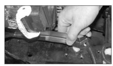
16. On 2002-2005 models slide the ABS pump inward to gain clearance for installation of the boot shield.
