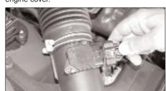
3. Disconnect the mass air electrical connection.
