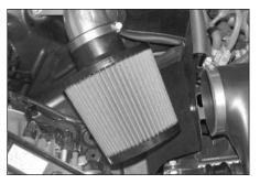
30. Install the  $K\&N^{\otimes}$  air filter and secure with the provided hose clamp as shown.
