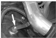
25. Secure the bracket to the rubber mounted stud using the provided hardware as shown.
