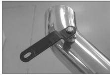
21. Secure the provided bracket to the K&N  $^{\! \otimes}$  intake tube using the provided hardware as shown.
