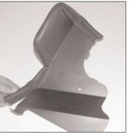
13. Install edge trim onto the heat shield as shown. Trim if needed.
