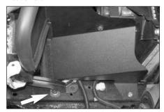
17. On 2002-2005 models install the heat shield and secure using the provided hardware.
