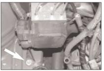
14. On 2001 models, loosen and remove the 12mm bolt that retains the ABS pump to vehicle.
