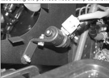
27. Mount the "L" bracket onto the heat shield and then mount the evap solenoid onto the bracket with the provided hardware.
