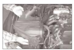
12. Remove the complete air box from vehicle. NOTE: K&N Engineering, Inc., recommends that customers do not discard factory air intake.
