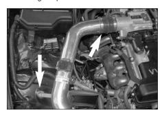
24. Slide the intake tube into the silicone hose, then, line up the bracket with the rubber mounted stud as shown.
