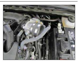
5. Install the provided coupler (08690) onto the throttle body and secure with the provided hose clamp.
