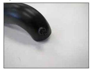
6. Install the provided vent fitting into the K&N® intake tube as shown.
