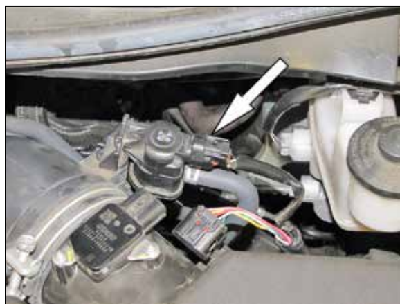
3. Disconnect the EVAP solenoid electrical connection.
