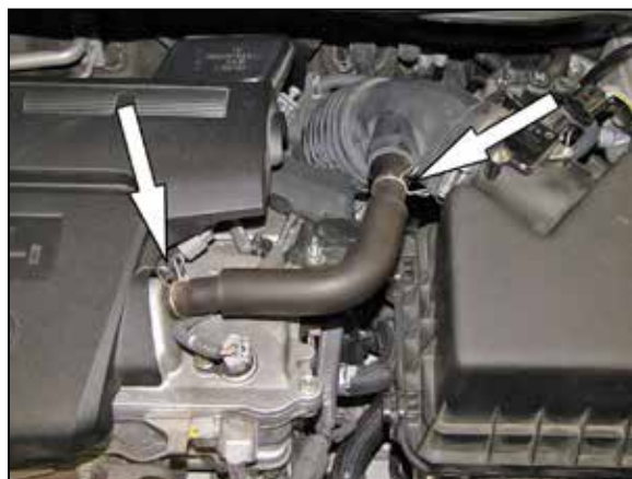
4. Release the spring clamps securing the Crank case vent hose and then remove the crank case vent hose from the vehicle.
