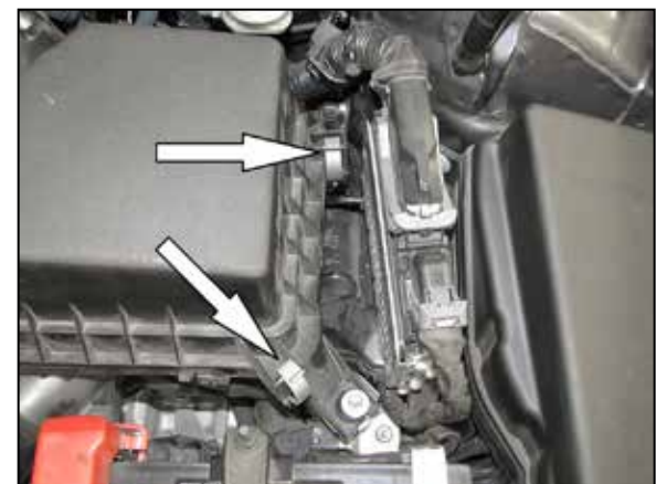
6. Release the two air box lid retaining clips and then remove the air box lid and factory air filter from the vehicle.
