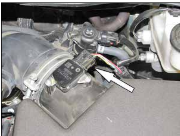
2. Disconnect the mass air sensor electrical connection.
