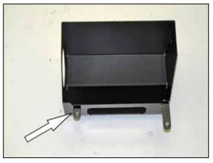
12. Install the provided "L" bracket (070066) onto the heat shield using the provided hardware.
