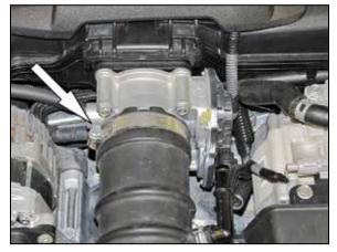
4. Loosen the hose clamp securing the intake hose to the throttle body.
