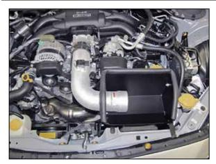
22. Rotate the tube down and install it into the silicone hose on the throttle body and install the mounting stud into the bracket. Secure the tube with the provided hose clamps and hardware and tighten the mounting bracket at this time.
