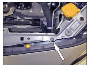
16. Remove the core support bolt shown. **NOTE: This bolt will be reused.**
