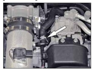
23. Connect the crank case vent to the fitting installed into the K&N<sup>®</sup> intake tube as shown.
