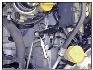
8. Install the provided heat shield mounting bracket (070026) onto the lower air box mount using the factory bolt.
