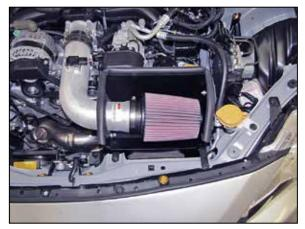
25. Install the K&N<sup>®</sup> air filter onto the K&N<sup>®</sup> intake tube and secure with the provided hose clamp. **NOTE: Drycharger<sup>®</sup> air ilter wrap; part # RC-4630DK is available to purchase separately.**
