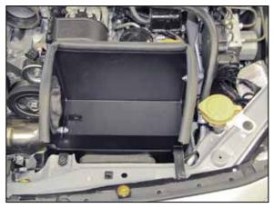
17. Set the heat shield into position on the core support and secure with the factory air box mounting bolts and to the previously install bracket with the hardware provided.
