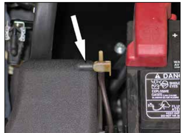
35. Install the provided vacuum plug onto the vacuum TEE.
