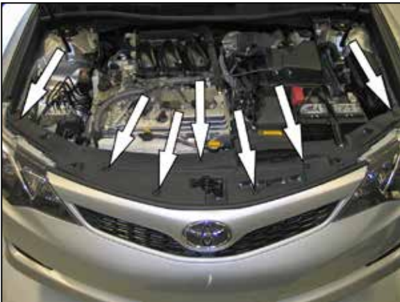
11. Remove the 7 clips securing the upper valance and then remove the upper valance from the vehicle.
