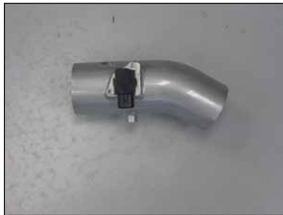
31. Install the mass air sensor into the K&N® intake tube and secure with the provided hardware.
