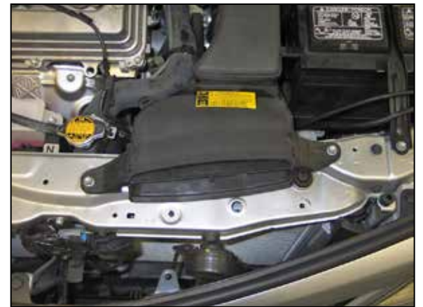
34. Reinstall the fresh air intake scoop and secure with the factory hardware.
