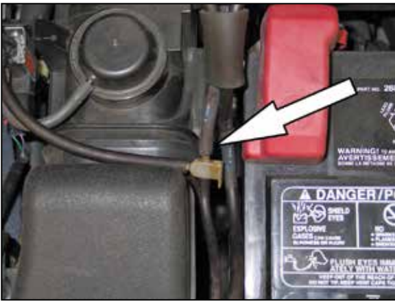
8. Disconnect the vacuum line at the TEE fitting shown.
