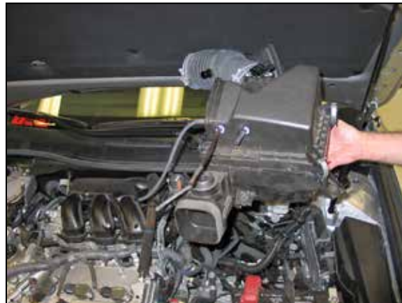
15. Remove the air box from the vehicle. NOTE: K&N Engineering, Inc., recommends that customers do not discard factory air intake.
