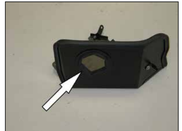
21. Install the 14.5" length edge trim into the hole of the heat shield as shown.
