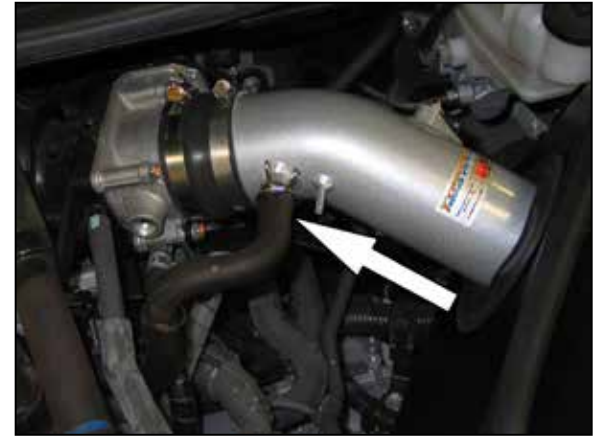
33. Connect the crank case vent hose to the K&N® intake tube and secure with the factory clamp.
