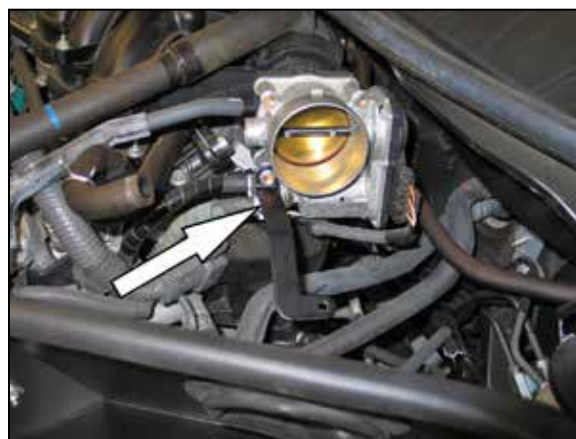
28. Install the tube mounting bracket (06485) onto the throttle body securing with the factory bolt removed in the previous step. NOTE: Do not completely tighten at this time.
