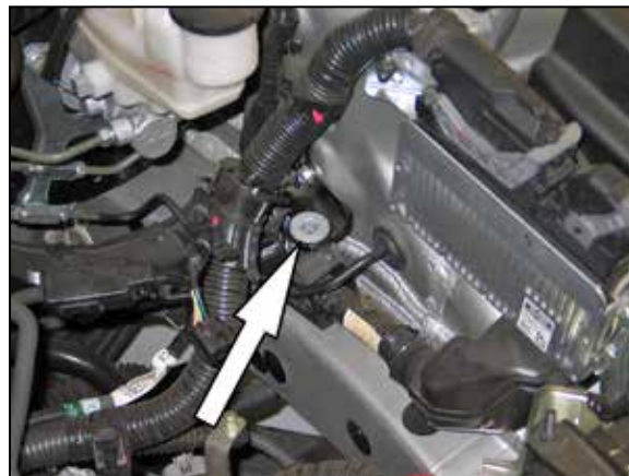
16. Remove the air box mounting grommet shown.
