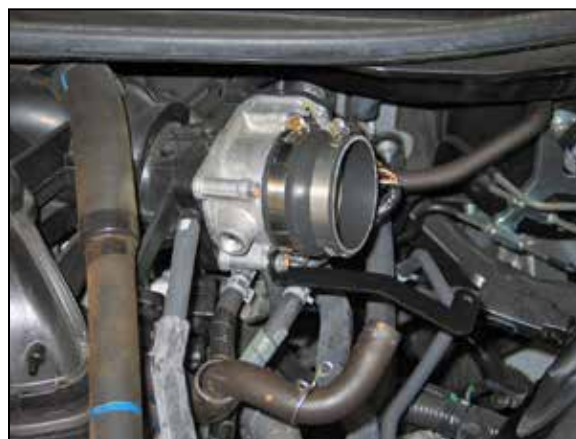
29. Install the silicone hose #084031 onto the throttle body and secure with the provided hose clamp.
