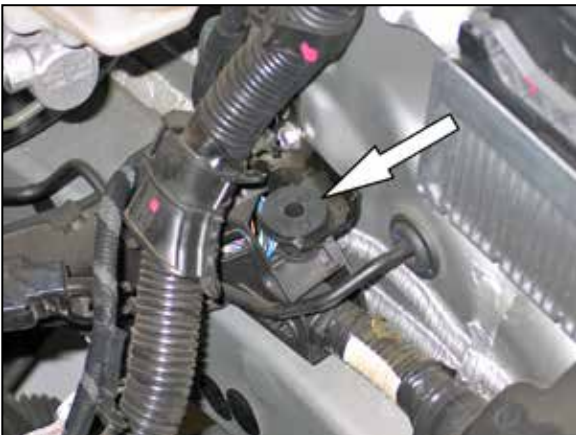
25. Install the provided inserted nut into the heat shield mounting bracket location.
