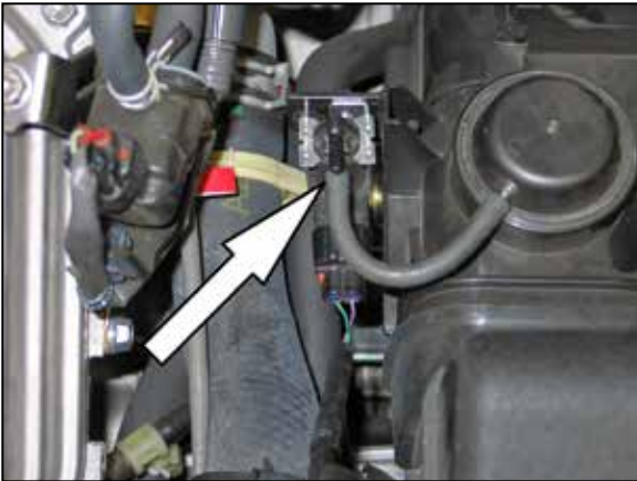
10. Disconnect the lower vacuum hose from the vacuum switching valve.
