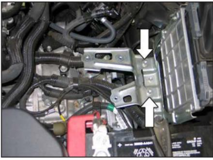
10. Remove the two air box mounting bracket bolts and then remove the bracket from the vehicle.
