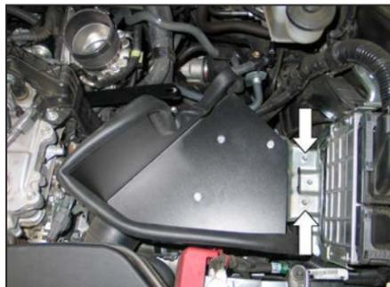
18. Install the heat shield assembly into the vehicle and secure with the factory air box mounting bracket bolts.
