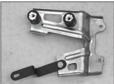
13. Install the heat shield mounting bracket (26655) onto the air box mounting bracket as shown.
