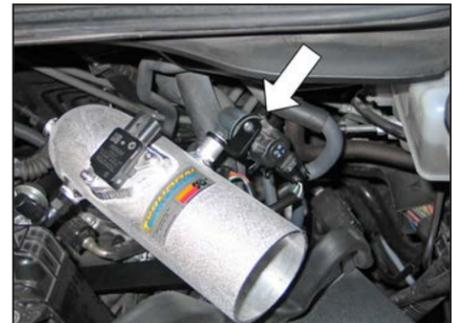
24. On vehicles equipped with EVAP valve, attach the EVAP solenoid to the bracket installed onto the K&N® intake tube and secure with the factory screw.
