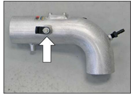
20. On vehicles equipped with EVAP valve, install the provided EVAP mounting bracket (070066) onto the K&N® intake tube using the provided hardware.
