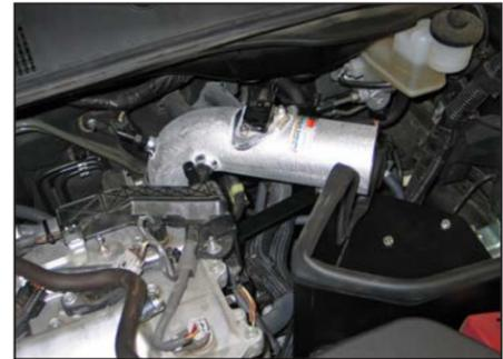
23. Install the K&N® intake tube into the silicone hose at the throttle body and align with the mounting bracket previously installed. Secure the tube with the provided hose clamp and hardware.
