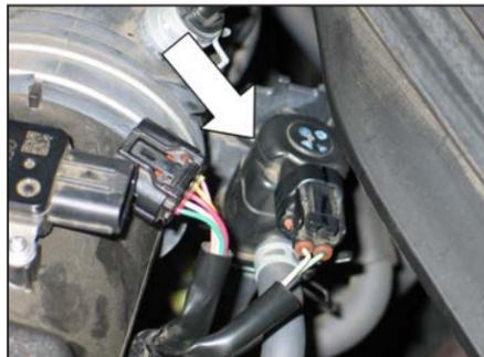
6. Lift up and remove the EVAP solenoid from the rear of the factory intake tube.
