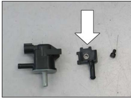
15. On vehicles equipped with EVAP valve, remove the EVAP control valve mounting bracket from the EVAP control valve.
