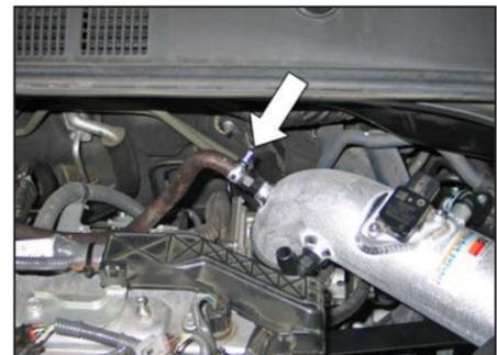
25. On vehicles equipped with EVAP valve, attach the EVAP vent line to the straight fitting installed in the K&N® intake tube.
