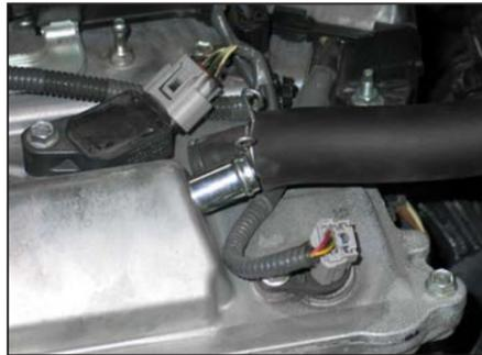
4. Disconnect the crank case vent hose from the valve cover as shown.
