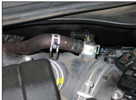
5. Disconnect the EVAP vent line from the factory intake tube as shown.
