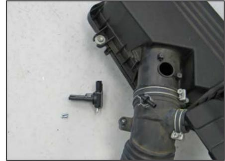
21. Remove the mass air sensor from the factory upper air box.
