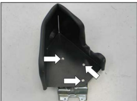
14. Attach the air box bracket assembly to the K&N® heat shield as shown using the provided hardware.
