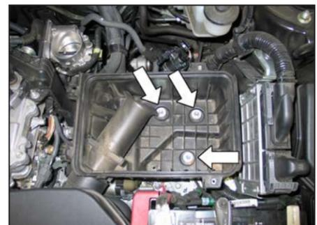
9. Remove the three lower air box mounting bolts and then remove the lower air box housing from the vehicle.
