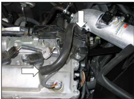
26. Attach the provided crank case vent hose to the 90° vent fitting in the K&N® intake tube and to the valve cover port as shown.
