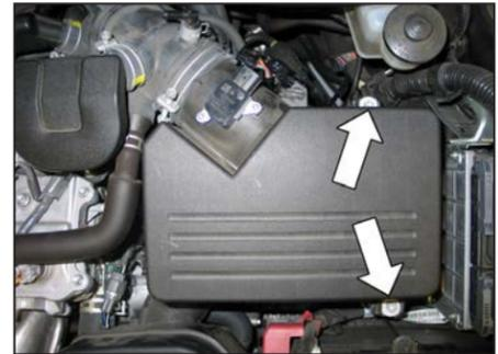
7. Loosen the two upper air box mounting bolts shown.
