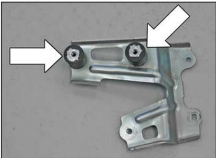
12. Install the two provided rubber mounted studs onto the factory air box bracket as shown.
