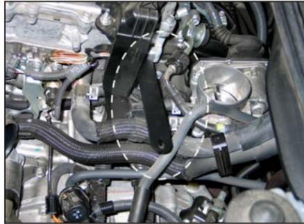
16. Install the tube mounting bracket (083162) onto the cylinder head as shown using the provided hardware.
