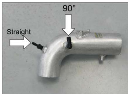
19. Install the two provided 1/4" NPT fittings into the K&N® intake tube as shown.
