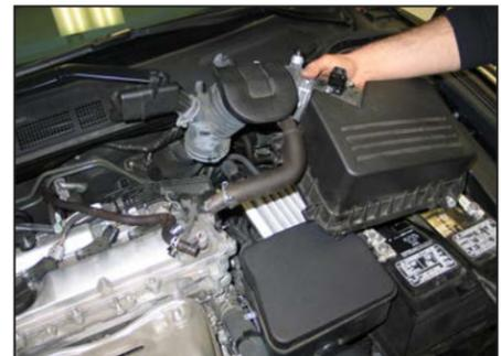
8. Loosen the hose clamp that secures the factory intake tube to the throttle body and then remove the intake tube and upper air box assembly.
