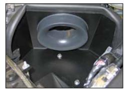
15. Install the filter adapter into the heat shield and secure with the provided hardware.
