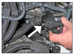
10. Remove the screw securing the EVAP solenoid mounting bracket and remove the mounting bracket.
