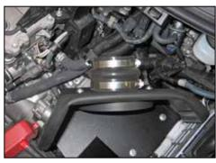
21. Install the provided silicone hose (087121) onto the filter adapter as shown.
