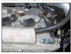
24. Connect the crank case vent hose to the valve cover port.
