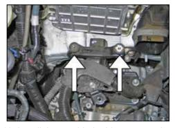
12. Install the provided rubber mounted studs (2) onto the air box mounting bracket as shown.
