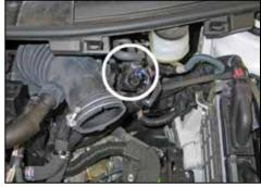
8. Unhook the EVAP solenoid from the intake tube.
