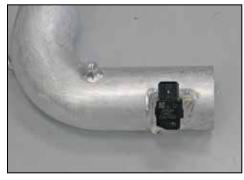
17. Install the mass air sensor into the K&N<sup>®</sup> intake tube and secure with the provided hardware.
