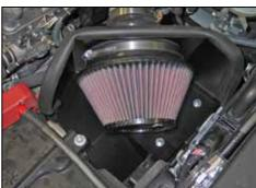
25. Install the K&N $^{\!0}$  air filter onto the filter adapter and secure with the provided hose clamp.
