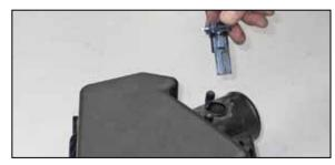
17. Remove the two screws that secure the mass air sensor to the stock air box. Then, remove the mass air sensor as shown.
