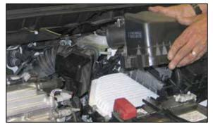
5. Loosen the hose clamp that secures the intake tube to the upper air box. Then, un-hook the three upper air box retaining clips. Remove the upper air box from the vehicle as shown.
