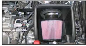
20. Install the K&N<sup>®</sup> air filter and secure with the provided hose clamp.
