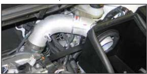
19. Install the intake tube into the silicone hose at the throttle body and align with the mounting bracket. Secure the EVAP bracket and mounting bracket in the same location on the intake tube using the provided hardware.
