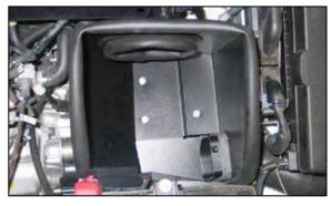
16. Install the heat shield assembly and secure with the provided hardware.
