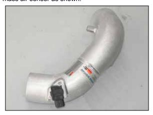
18. Install the mass air sensor into the intake tube and secure with the provided hardware as shown.
