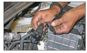
8. Un-hook the EVAP wiring harness from the EVAP mounting bracket as shown.
