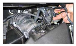
4. Un-hook the EVAP solenoid valve from the stock intake tube as shown.
