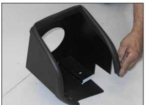
14. Install the long edge trim onto the heat shield as shown.
