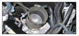
12. Install silicone step hose (#08713) onto the throttle body and secure with the provided hose clamp.
