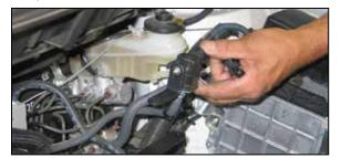
13. Install the provided EVAP bracket onto the EVAP solenoid with the provided hardware.
