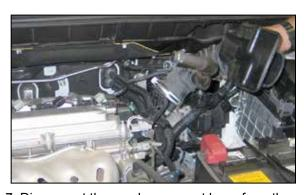
7. Disconnect the crank case vent hose from the valve cover. Loosen the spring clamp that secures the intake tube to the throttle body and remove the stock intake tube from the vehicle.
