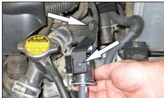
21. Remove the screw that secures the vacuum switching valve to the bracket. Un-clip the wiring harness from the bracket as shown.
