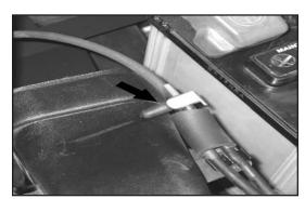
27. Install one vacuum cap plug onto the the factory "T" fitting as shown in the photograph.
