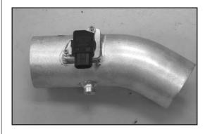
22. Install the mass air sensor removed in the previous step into the K&N<sup>®</sup> intake tube and secure with the provided hardware.
