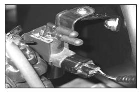
26. Install the two vacuum cap plugs onto the "vacuum switching valve."
