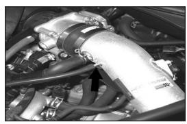
30. Install the supplied vacuum hose to the  $K\&N^{\otimes}$  Intake Tube.
