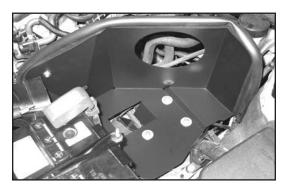
17. Place the heat shield into position, aligning the front mounting hole with the rubber mounted stud installed in step #14. Secure the heat shield to the air box mounting bracket using the hardware provided.
