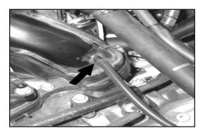
29. Connect the open end of the vacuum line installed in the previous step to the intake manifold plenum connection.
