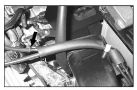
31. Connect the open end of the vacuum line installed in the previous step to the stock fitting as shown in the photograph.
