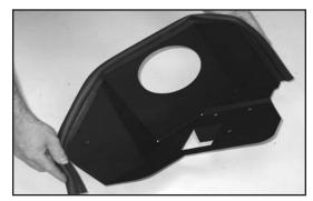
15. Install the edge trim onto the heat shield. Note: Some trimming of the edge trim may be necessary.
