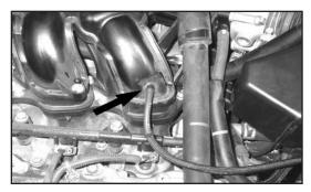
4. Disconnect the vacuum line from the intake manifold plenum connection.
