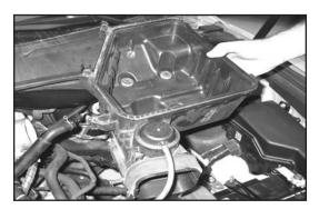
13. Remove the lower air box from the vehicle. NOTE: K&N Engineering, Inc., recommends that you do not discard your factory air intake.
