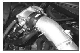
25. Connect the crank case vent hose to the fitting on the  $K\&N^{@}$  intake tube; secure with the factory spring clamp.
