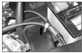
28. Install the supplied vacuum hose onto the factory "T" fitting as shown in the photograph.
