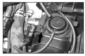
9. Remove the screw securing the "Vacuum switching valve" to the stock fresh air duct. Place the "Vacuum switching valve" in a position that will allow ample clearance to work around.
