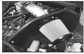
32. Install the K&N  $^{\! 8}$  air filter onto the K&N  $^{\! 8}$  intake tube; secure with the provided hose clamp.
