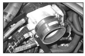
20. Install the provided silicone hose (084031) onto the throttle body and secure with the provided hose clamp.
