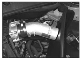
23. Install the K&N<sup>®</sup> intake tube into the silicone hose installed onto the throttle body in step # 20. Align the K&N<sup>®</sup> intake tube with the intake tube mounting bracket installed in step # 19. Secure silicone hose with provided hose clamp and mounting bracket with provided hardware.
