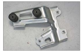
18. Install the two rubber mounted studs onto the air box mounting bracket as shown.
