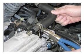
11. Using a pair of pliers, loosen the hose clamp that secures the crank case vent hose to the valve cover; then, disconnect the crank case vent hose from the valve cover.
