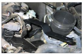
16. Install the intake tube mounting bracket (26654) onto the engine using the provided hardware. Note: The bracket will fasten to the threaded boss at the rear corner of the cylinder head.
