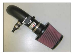
30. Install the air filter onto the intake tube secure using the provided hose clamp. NOTE: Drycharger<sup>®</sup> air ilter wrap; part # RX-4990DK is available to purchase separately.
