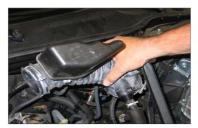
12. Using a pair of pliers, loosen the hose clamp that secure the stock intake tube to the throttle body; then, remove the intake tube from the throttle body as shown in the photograph.
