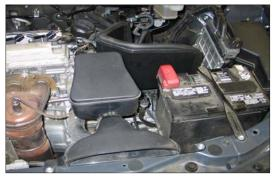
22. Install the fresh air intake onto the provision on the heat shield and adjust for proper fit; then, fasten with the stock bolts removed in step #5.
