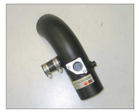
26. Install the provided silicone hose (084074) onto the intake tube and secure with the provided hose clamp.
