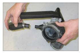
24. Release the hose clamp and remove the crank case vent hose from the crank case vent chamber as shown in the photograph.
