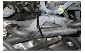
14. Using the provided tie-wrap, secure the heater hoses to the throttle body bypass hoses as shown in the photograph.
