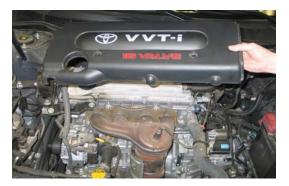
10. Remove the two nuts that secure the engine cover; then, remove the engine cover from the vehicle and set aside.
