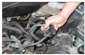
13. Position the intake tube in a fashion that will allow access to the Pulse width modulated (PWM) switching valve mounting screw; then remove the screw. Remove the entire intake tube assembly from the vehicle.
