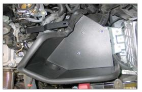
21. Place the heat shield into position and secure the air box mounting bracket to its original location using the two stock bolts removed in step #9.
