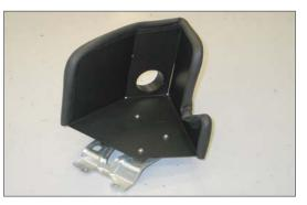
20. Install the air box mounting bracket assembly onto the heat shield and secure with the provided hardware.
