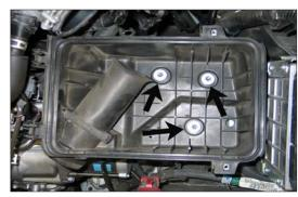
7. Remove the three bolts that secure the lower air box to the mounting bracket.
