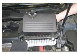
4. Remove the air box lid from the vehicle.
