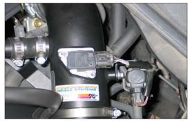
35. Re-connect the mass air sensor electrical connection.
