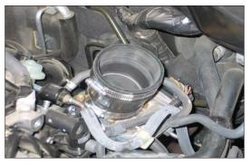
15. Install the provided silicone step hose (08095) onto the throttle body and secure with the provided hose clamp.
