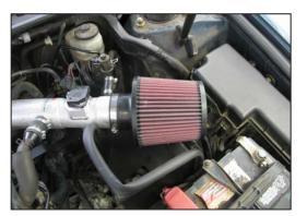
25. Install the K&N<sup>®</sup> air filter onto the intake tube; secure with the provided hose clamp.
