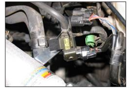
13. Install the intake tube mounting bracket (26651) onto the engine using the provided hardare as shown in the photograph.
