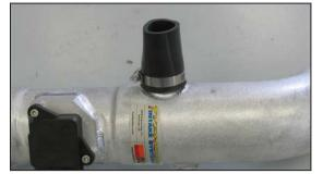
17. Install the provided silicone hose (084074) onto the K&N^ $^{\scriptsize (\!R\!)}$  intake tube and secure with the provided hose clamp.
