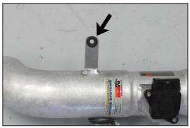
20. Install the provided grommet into the welded bracket on the K&N $^{\mbox{${\rm R}$}}$  intake tube.
