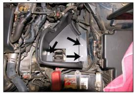
12. Set the heat shield into position on the lower air box mount and inner fender. Using the provided hardware, secure the heat shield to the three original lower air box mount's threaded holes.
