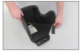
10. Install the provided edge trim onto the heat shield as shown in the photograph. NOTE: Some trimming of the edge trim may be necessary.
