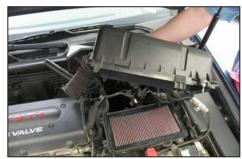
6. Release the clamp that secures the stock intake tube to the throttle body. Then, remove the factory intake tube/upper air box as shown in the photograph.
