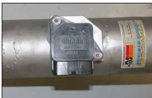
20. Install the mass air sensor into the K&N® intake tube and secure with the provided hardware as shown.
