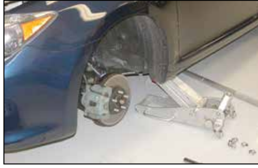
15. Raise the vehicle up and support it with jack stands, then, remove the front tire as shown.
