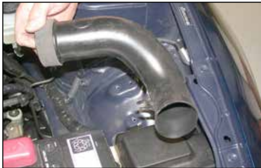
12. Remove the air inlet duct as shown.
