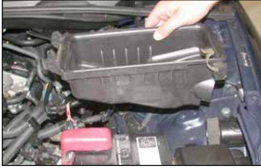
11. Remove the lower air cleaner assembly as shown. NOTE: K&N Engineering, Inc., recommends that customers do not discard factory air intake.
