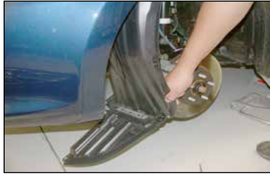
16. Remove four screws and three plastic rivets, then, pull the inner fender valance downward as shown.
