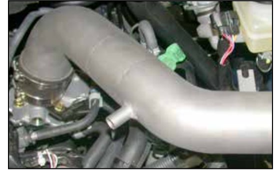
22. Slide the K&N® intake tube into the silicone hose on the throttle body as shown.
