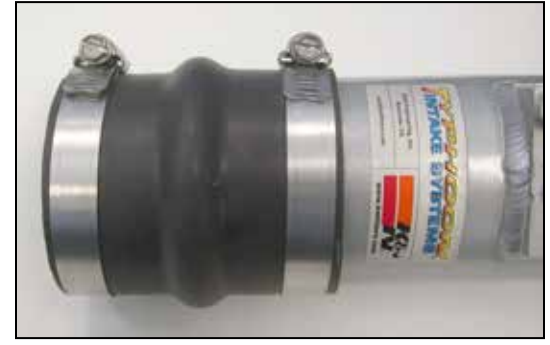
21. Install the provided silicone hump hose and hose clamps onto the K&N® intake tube and secure as shown.
