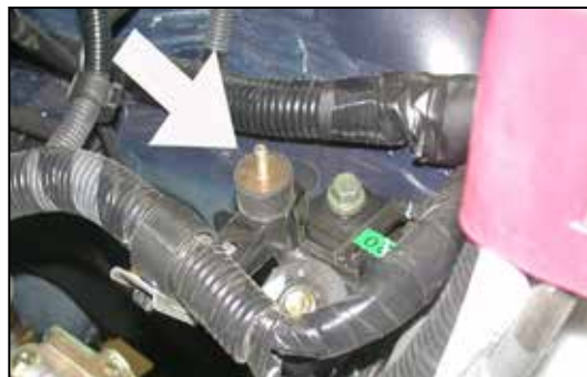
18. Install the rubber mounted stud into the original air cleaner mounting hole as shown.
