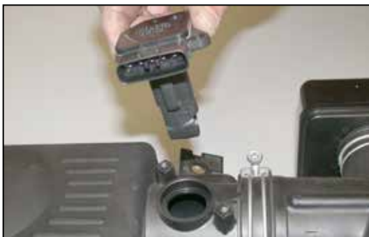
14. Remove the mass air sensor from the air cleaner as shown.
