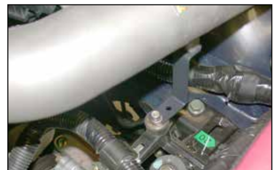
23. Secure the bracket to the rubber mounted stud using the provided hardware but do not tighten at this time.
