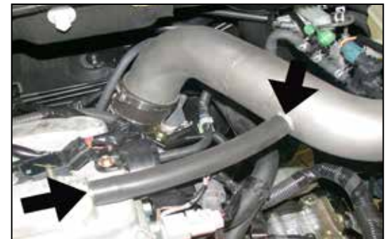
25. Slide the provided hose onto the cam cover, then, connect the other end to the vent on the K&N® intake tube as shown.
