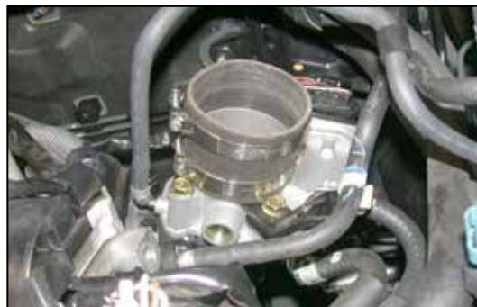
17. Install the silicone hose and hose clamps onto the throttle body as shown.
