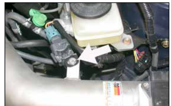
24. Secure the vacuum switching valve to the bracket on the K&N® intake tube using the provided hardware as shown.
