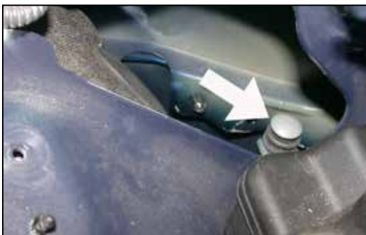
13. Remove the air inlet duct screws from the inner fender as shown.
