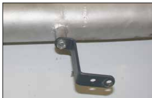
19. Install the provided bracket onto the K&N® intake tube and secure with the provided hardware, but do not tighten completely at this time. NOTE: Before installing the bracket, inspect the inside of the tube for any debris, then clean the inside out with water and a towel. Inspect the tube one more time before proceeding to the next step.
