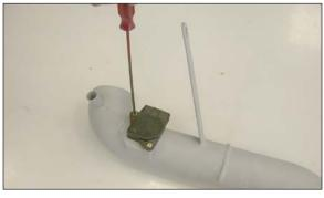
25. Install the stock mass air sensor into the K&N $^{\odot}$  cold air tube and secure with the provided hardware as shown.
