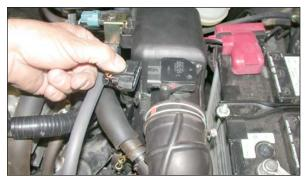
3. Disconnect the mass air sensor electrical connection as shown.
