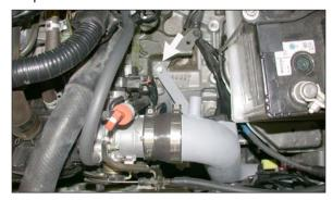
27. Slide the end of the tube into the silicone hose on the throttle body, then secure the bracket to the air cleaner mounting hole using the provided hardware as shown but do not tighten at this time.
