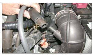
7. Disconnect the crank case vent hose from the stock intake tube as shown.
