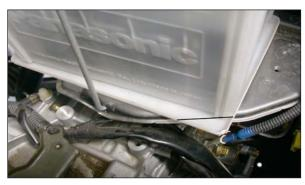
16. Using a cutting tool, trim the plastic battery tray to mirror the inner fender as shown.
