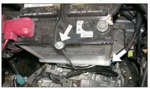
15. Loosen the battery hold down bracket and slide the battery as far towards the fender as possible.
