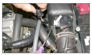
4. Using a flat blade screwdriver unclip the wire harness as shown.
