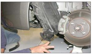
20. Remove the two bolts that secure the inner fender valance, then, lower the valance downward
