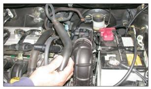
9. Disconnect the crank case vent hose from the cam cover, then, remove the crank case vent hose as shown.
