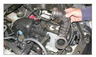
10. Loosen the hose clamps at the throttle body and at the air cleaner assembly, then, remove the stock intake tube as shown.
