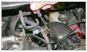
6. Use a flat blade screwdriver to unclip the vacuum switching valve from the side of the air cleaner assembly as shown.
