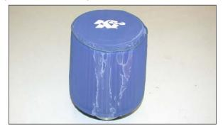
31. Install the Drycharger® onto the K&N $^{\mbox{\tiny B}}$  air filter as shown.
