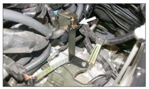
22. Slide the vacuum switching valve onto the "L" bracket as shown.
