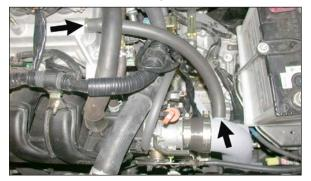
30. Install the provided silicone hose onto the vent on the K&N<sup>®</sup> intake tube, then, connect the other end to the vent on the cam cover along with the provided hose clamp.
