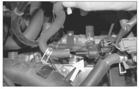
24. Remove the vent hose from the EVAP OBD canister closed valve as shown.
