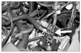
23. Slide the PWM vacuum switching valve onto the T-bracket as shown.
