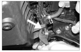
11. Using a pair of pliers unclip the wire harness from the lower air cleaner assembly as shown.
