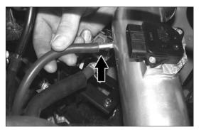
32. Connect the EVAP OBD canister closed value to the vent on the K&N $^{\circ}$  Typhoon $^{\circ}$  intake tube as shown.
