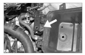
12. Remove the bolt that secures the EVAP OBD canister closed valve to the lower air cleaner assembly as shown.
