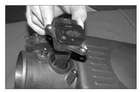
26. Remove the mass air sensor from the upper air cleaner assembly as shown.
