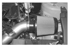
33. Install the K&N X-Stream air filter onto the K&N<sup>®</sup> Typhoon intake tube as shown.
