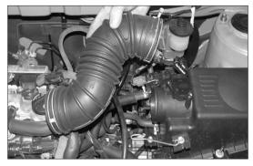
6. Loosen the hose clamps at the throttle body and at the air cleaner, then, remove the stock intake tube as shown. 8. Unclip the upper air cleaner assembly and tilt it upward, then, using a flat blade screwdriver depress the release tab on the air cleaner assembly to release the PWM vacuum switching valve as shown.
