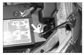
15. Remove the bolt that secures the air inlet duct to the inner fender as shown.
