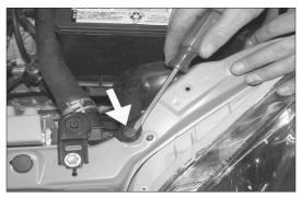
16. Remove the push clip that secures the air inlet duct to the radiator core support as shown.
