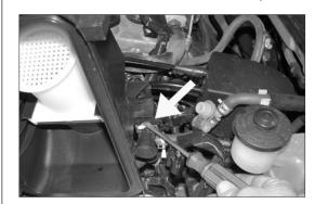
2. Using a flat blade screwdriver remove the two push clips on the engine cover as shown. Also remove the two acorn nuts on the engine cover.
