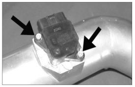
27. <u>Install the mass air sensor</u> into the K&N<sup>®</sup> Typhoon<sup>®</sup> intake tube using the provided hardware as shown.
