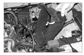
13. Remove the lower air cleaner assembly as shown.
