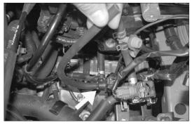
25. Install the provided silicone hose onto the EVAP OBD canister closed valve as shown.
