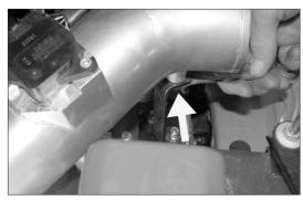
30. Line up the K&N<sup>®</sup> Typhoon<sup>®</sup> intake tube with the "C" bracket and adjust the bracket for best fit, then, secure the tube to the bracket with the provided hardware.
