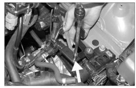
20. Secure the EVAP OBD canister closed valve to the T-bracket from step 19 using the provided hardware.
