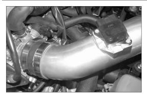
29. Slide the K&N<sup>®</sup> Typhoon intake tube into the silicone hose on the throttle body as shown. Do not tighten completely at this time.
