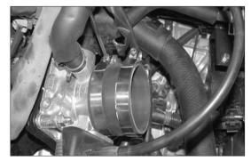
28. Install the silicone hose and hose clamps onto the throttle body and secure as shown.
