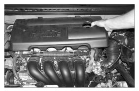
3. Remove the engine cover as shown.
