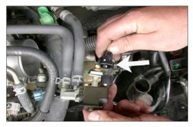
18. Disconnect the PWM vacuum switching valve electrical connection as shown.
