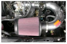
42. Install the air filter onto the intake tube and secure with the provided hose clamp as shown.
