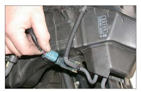
14. Disconnect the vacuum switching valve
