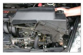
17. Remove the complete air cleaner assembly as shown.
