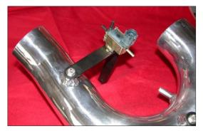
27. Secure the "L" bracket to the threaded boss on the Typhoon intake tube using the provided hardware as shown.
