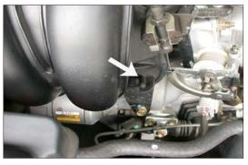
41. Cap the vent on the intake manifold using the provided rubber plug as shown.
