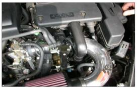
44. Install the computer fresh air tube as shown.
