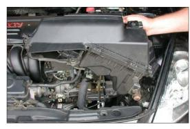
12. Push back, and pull up to gain access to the bottom of the air cleaner assembly as shown. NOTE: K&N Engineering, Inc., recommends that customers do not discard factory air intake.
