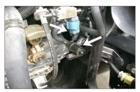
38. Reconnect the EVAP OBD canister closed valve
