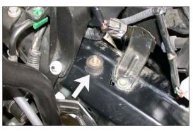
34. Install the provided rubber mounted stud into the existing air cleaner mounting hole as shown.
