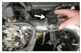
35. While sliding the intake tube into the silicone hose on the throttle body, reconnect the mass air sensor electrical connection as shown.
