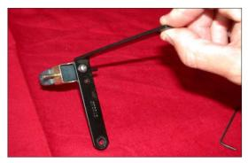
25. Secure the vacuum switching valve to the provided "L" bracket using the provided hardware as shown.
