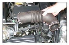
9. Loosen the hose clamps on the stock intake tube, then, remove the stock intake tube as shown.
