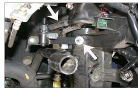
31. Install the EVAP OBD canister closed valve assembly into the vehicle and connect the hose to the hard line, then, secure the bracket to the relay and fuse box support bracket using the nut removed in step 29.
