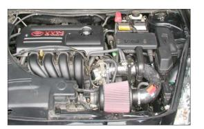
46. Reconnect the vehicle's negative battery cable. Double check to make sure everything is tight and properly positioned before starting the vehicle.
