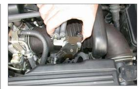
7. Unclip the PWM vacuum switching valve from the rear of the air cleaner assembly as shown.
