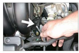
13. Remove the vacuum hose from the intake manifold as shown.
