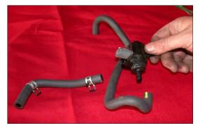
23. Remove the two vent hoses from the EVAP OBD canister closed valve as shown.
