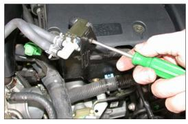
19. Remove the stock bracket from the PWM vacuum switching valve as shown.
