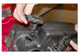
20. Remove the mass air sensor from the air cleaner assembly as shown.
