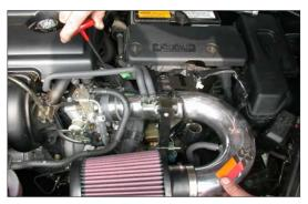
43. Adjust the tube for best fit and clearance and tighten all hardware and hose clamps as shown.
