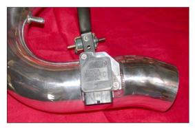
28. Install the mass air sensor into the intake tube and secure using the provided hardware as shown.
