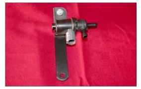
24. Secure the EVAP OBD canister closed valve to the provided angle bracket using the provided hardware as shown.
