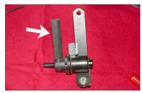
30. Connect the provided silicone hose onto the EVAP OBD canister closed valve as shown.
