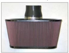
17. Install the provided silicone hose (084055) onto the K&N<sup>®</sup> air filter and secure with the provided hose clamp.
