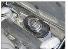
18. Set the K&N<sup>®</sup> filter assembly into position on the radiator shroud as shown.
