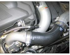
20. Connect the crank case vent fitting to the fitting on the K&N $^{\mbox{\tiny @}}$  intake tube.
