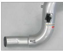
16. Install the mass air sensor into the K&N<sup>®</sup> intake tube and secure it with the provided hardware.
