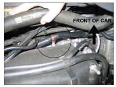
13. Unhook the engine wiring harness from the stud on the front of the engine.
