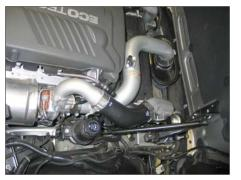
10 Install the KRN® intake tube into the silicone
