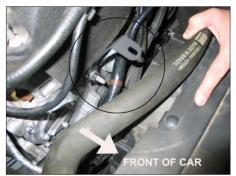
14. Install the tube mounting bracket (083122) onto the stud on the front of the engine and secure with the hardware. Re-secure the wiring harness to the stud after the bracket has been installed.
