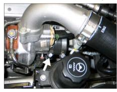
12. Install the silicone hose (08476) onto the turbo inlet and secure with the provided hose clamp.
