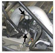
11. Reinstall the left side intercooler tube mounting bracket and secure with the factory hardware.
