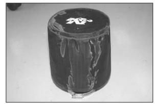
25. Slide the K&N® Drycharger® onto the K&N® air filter as shown.
