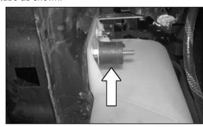
20. Install the provided washer and the provided rubber mounted stud onto the lower bolt on the windshield wiper reservoir as shown.
