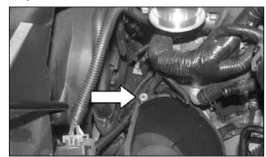
16. Place the provided spacer onto the front mounting point of the original air cleaner cover as shown.
