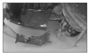
12. Remove the four plastic rivets, then, remove the plastic valance as shown.
