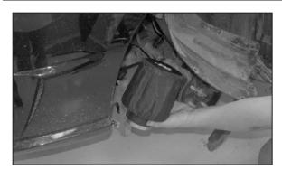
26. From underneath the vehicle slide the K&N® air filter onto the K&N® intake tube as shown.
