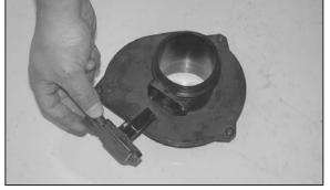
7. Remove the mass air sensor from the air cleaner cover as shown.
