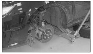
10. Jack the vehicle up and support it with jack stands, then, remove the front driver side tire as shown.
