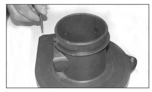
8. Remove one of the stock screws as shown because this will be re-used at a later time.
