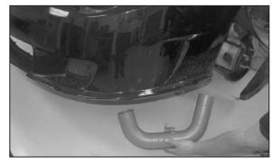
23. From underneath the vehicle slide the K&N® cold air tube up into the inner fender as shown.
