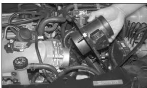
4. Loosen the three screws to remove the stock air cleaner cover as shown.
