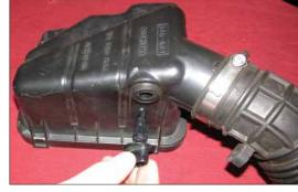
8. Remove the air temperature sensor from the upper air cleaner assembly as shown.
