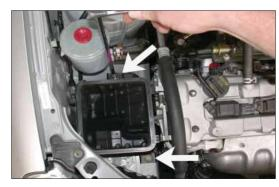
Remove the two bolts that secure the lower air cleaner assembly.
