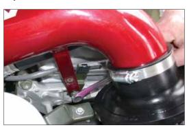
15. Line up the bracket with the threaded hole from step 9 and secure with the stock bolt from step 9.
