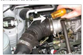
3. Loosen the hose clamp at the throttle body as shown.
