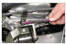
9. Remove the bolt that secures the wire harness bracket to the engine mount bracket as shown.
