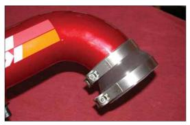
12. Install the silicone hose and hose clamps onto the intake tube as shown.
