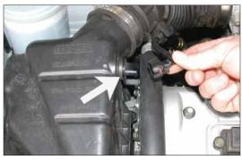
2. Disconnect the air temperature sensor electrical connection as shown
