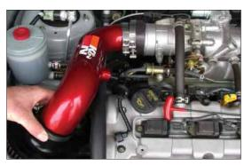
14. Install the intake tube assembly onto the throttle body as shown.
