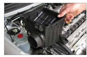
7. Remove the lower air cleaner assembly as shown.
