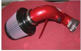
13. <u>Install the air fitler on to the intake tube</u> as shown.
