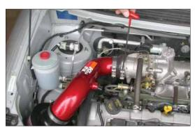
16. Tighten the hose clamp on the throttle body as shown.
