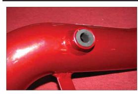
10. Install the silicone hose into the vent on the Typhoon intake tube as shown.
