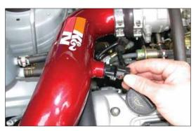
17. Reconnect the air temperature sensor electrical connection as shown.
