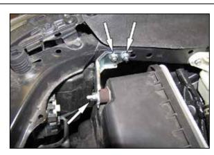
5. Remove the three nuts that secure the air filter housing to the inner fender and then remove the bracket from the vehicle.
