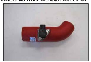
11. Remove the mass air sensor from the factory air filter housing and install it into the K&N<sup>®</sup> intake tube using the provided hardware.
