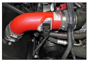
15. Reconnect the mass air sensor electrical connection.
