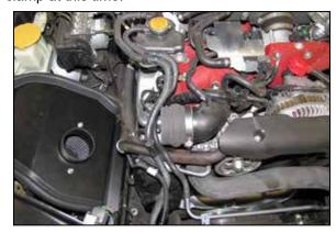
13. Install the provided hump coupler (08185) onto the turbo inlet tube. Set the heat shield assembly into position on the inner fender but do not secure.
