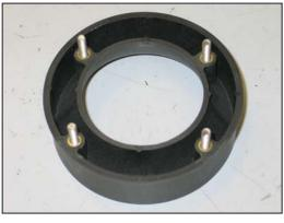
11. Install the four 6mm studs into the filter adapter as shown.
