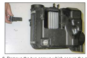
8. Remove the two screws which secure the mass air sensor and then remove the mass air sensor from the airbox as shown.
