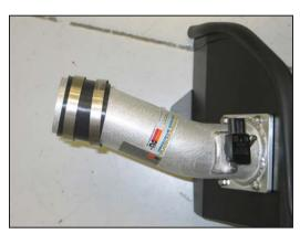
16. Install the provided silicone hose (08440) onto the intake tube as shown.
