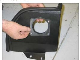
13. Install the filter adapter assembly into the heat shield and then install the remaining gasket onto the studs protruding through the heat shield as shown.
