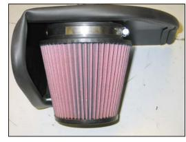
15. Install the K&N® air filter onto intake assembly and secure with the provided hose clamp.
