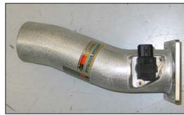
9. Install the mass air sensor into the K&N® intake tube and secure with the provided hardware.
