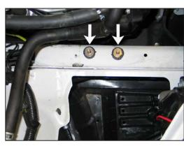
7. Install the two rubber mounted studs into the inner fender as shown.
