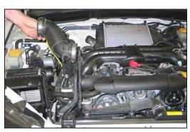
4. Loosen the two hose clamps which secure the factory intake tube and then remove the intake tube from the vehicle.
