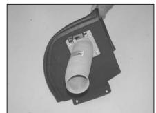
15. Install the intake tube onto the studs and secure with two of the provided nylock nuts and flat washers as shown in the orientaion.
