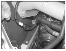
24. Zip-tie the coolant hose and power steering hose together as shown.
