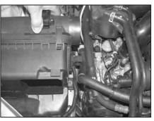
8a. Pull the air cleaner upwards and unclip the coolant hose and the mass air sensor wire harness from the side of the air cleaner.
