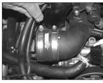
17. Install the provided silicone hose and hose clamps onto the turbo inlet tube as shown.
