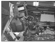
8b. Then remove the air cleaner as shown. NOTE: K&N Engineering, Inc., recommends that customers do not discard factory air intake.
