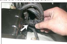
22. Unclip the wire harness from the inner fender bracket as some slack will be needed to reroute the mass air sensor electrical connection.
