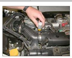
5. Loosen the hose clamp on the turbo charger inlet tube as shown.
