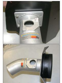
10. Assemble the tube, heat shield, filter adapter, and the remaining gasket using two of the provided hex bolts as shown above.
