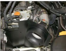
16. Install the complete air cleaner assembly into the vehicle and slide the intake tube into the silicone hose as shown above.
