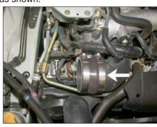
8. Install the silicone hose and hose clamps onto the turbo charger inlet tube as shown.
