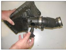
7. Remove the mass air sensor from the air cleaner as shown.
