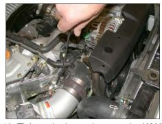
18. Tighten the hose clamp on the  $K\&N^{\otimes}$  intake tube as shown.
