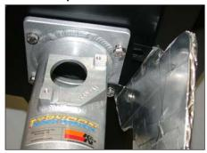
11. Using the remaining hex bolts install the heat deflector plate onto the intake tube flange as shown.
