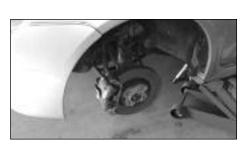
10. Taking the necessary safty precautions raise the front of the vehicle and support it with axle stands. Now remove the L/H front wheel as shown.
