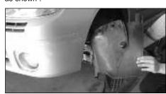
11. Remove the L/H wheel arch liner.
