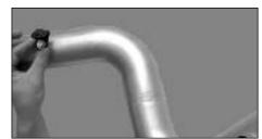
14. Fit the bracket onto the threaded standoff on the new intake pipe using the M6 bolt and M6 waved washer supplied. (do not fully tighten yet.)
