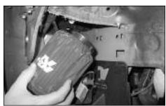
20. Fit the filter on to the intake pipe using the #44 hose clamp supplied. Align the complete intake tube assembly for maximum clearance. Now firmly tighten all hose clamps and hard-
