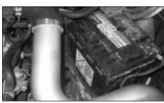
22. Re-install the battery to the vehicle and reconnect the battery terminals (positive terminal first).
