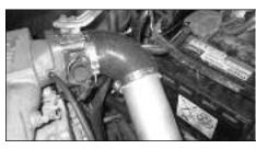
23. Re-install the ECU mounting bracket using its original hardware.
