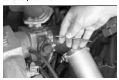
18. Fit the silicone hose on to the throttle housing using the #44 hose clamp supplied. Don't fully tighten yet!
