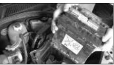
8. Disconnect first the negative, then the positive cable from the battery & remove the battery from the vehicle.
