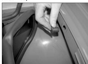
24. Install the threaded insert into inner fender as shown.
