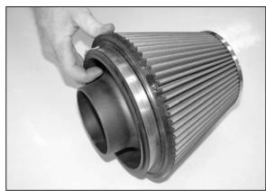
19. Install the filter adapter into the K&N® filter as shown. Secure with the provided hose clamp. NOTE: Drycharger® air filter wrap; part # 22-8049DK is available to purchase separately.
