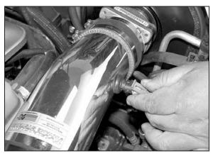
31. Reconnect the temperature sensor electrical connection.
