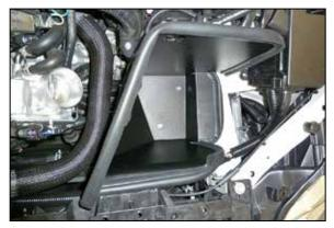
12. Install the heat shield into the vehicle so the mounting studs insert into the factory mounting grommets then secure the heat shield and wiring harness with the hardware provided.
