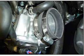
13. Install the provided coupler (08186) onto the throttle body and secure with the provided hose clamp.
