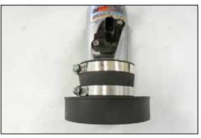
15. Remove the mass air sensor from the factory housing and then install it into the K&N<sup>®</sup> intake tube and secure with the provided hardware. Install the coupler (084036) onto the K&N<sup>®</sup> intake tube and then install the filter adapter into the coupler and secure them with the provided hose clamp.
