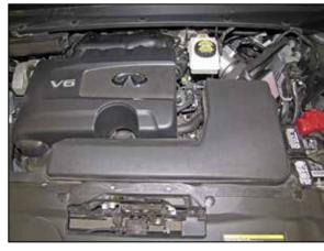
19. Reinstall the fresh air duct so it inserts slightly into the K&N® heat shield then secure with the factory hardware.
