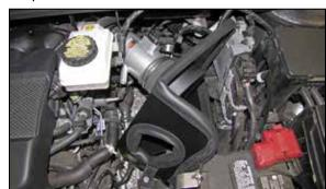
15. Install the heat shield assembly into the vehicle so the mounting studs insert into the factory air filter housing mounting studs and the intake tube inserts into the coupling hose. Secure the heat shield with the provided hardware then adjust the intake tube for best fit and secure with the provided hose clamps.
