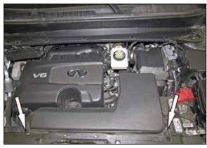
2. Remove the two bolts that secure the fresh air duct and then remove the fresh air duct from the vehicle.
