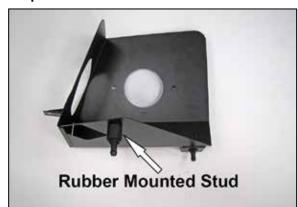
10. Install the heat shield mounts and rubber mounted stud onto the heat shield as shown.
