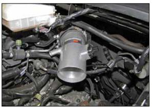
9. Install coupler hose (08690) onto the throttle body and secure with the provided hose clamp. Then install the  $K\&N^{\otimes}$  intake tube into the coupling hose as shown.
