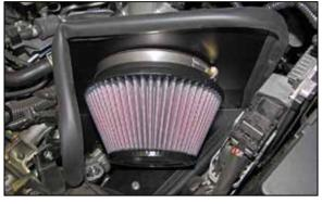
18. Install the K&N® air filter onto the adapter and secure with the provided hose clamp.
