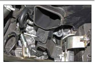
5. Remove the bolt which secures the air filter housing to the mount.
