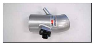
8. Remove the mass air sensor from the factory air box and then install it into the K&N® intake tube and secure with the provided hardware.
