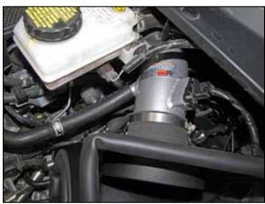
17. Install the hose mender into the factory crank case vent hose and secure with the factory spring clamp then connect the open end of the hose to the port on the K&N® intake tube.
