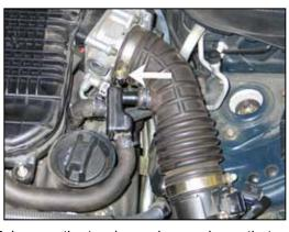
5. Loosen the two hose clamps shown that secure the driver's side intake tube.
