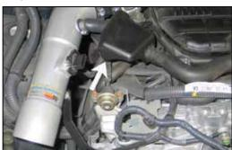
45. Connect the crankcase vent hose to the K&N<sup>®</sup> intake tube and secure with the provided hose clamp. Secure the crankcase vent chamber with the factory bolt removed during step #30.
