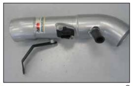
43. Install the mass air sensor into the K&N<sup>®</sup> intake tube and secure with the provided hardware.
