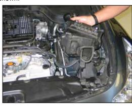
9. Remove the driver's side airbox assembly from the vehicle.
