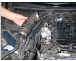
33. Remove the stock intake tube as shown.
