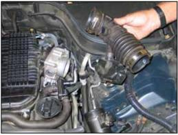
6. Release the spring clamp which secures the crankcase vent hose to the intake tube and then remove the intake tube from the vehicle.
