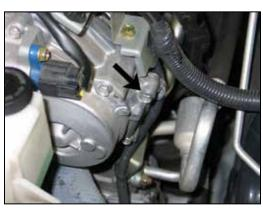
12. Remove the cam cover bolt shown.
