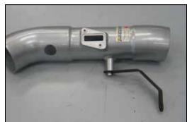
17. Attach the tube mounting bracket (07171) onto the driver's side intake tube (27412) using the supplied hardware.
