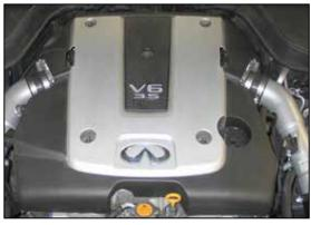
52. Install the engine cover and secure with the factory mounting hardware.
