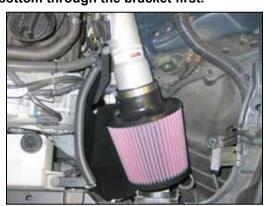
28. Install the  $K\&N^{\textcircled{R}}$  air filter onto the intake tube as shown and secure with the provided hose clamp
