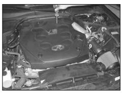
20. Reinstall the engine cover and the air inlet duct as shown.
