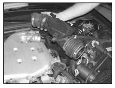
5. Remove the stock intake tube as shown.
