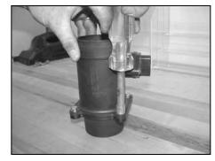
3. Disconnect the crankcase vent hose as shown.
