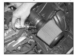
17. Install the K&N<sup>®</sup> air filter and secure with the provided hose clamp as shown. NOTE: Drycharger<sup>®</sup> air filter wrap; part # RX-4990DK is available to purchase separately.
