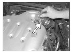
12. Install the provided silicone hose and hose clamps onto the throttle body and tighten.
