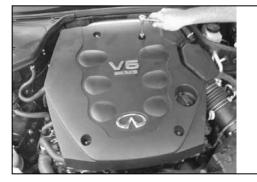
2. Remove the engine cover as shown.
