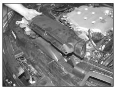
8. Disengage the two plastic rivets, then, remove the stock air inlet duct as shown.
