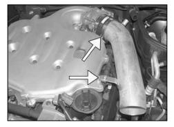
13. Install the K&N<sup>®</sup> intake tube into the silicone hose on the throttle body, then, line up the tube bracket with the threaded hole on the intake manifold and secure it with the bolt from step 4. **NOTE: Before installing the intake tube, inspect** the inside of the tube for any debris, then clean the inside out with water and a towel. Inspect the tube one more time before proceeding to the next step.
