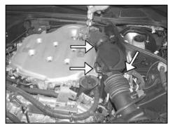
4. Loosen the hose clamps at the throttle body and at the mass air sensor, then, loosen and remove the bolt that secures the resonator to the intake manifold. 7. Unclip the air cleaner lid, then, loosen and remove the single bolt that secures the air cleaner lid to the fender. Rotate the air cleaner lid, then, unclip the mass air sensor electrical connection to remove the air cleaner lid as shown.
