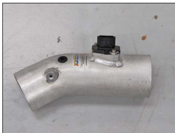
16. Install the mass air sensor into the K&N® intake tube and secure with the provided hardware.
