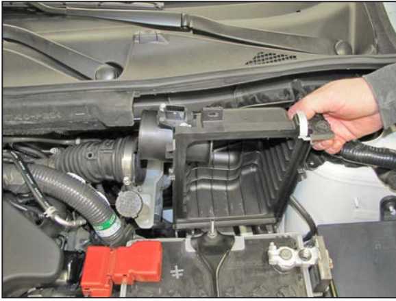
7. Lift up the rear air box housing and remove it from the vehicle.
