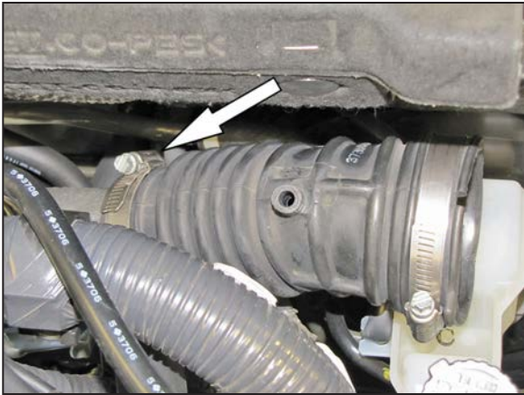
8. Loosen the hose clamp securing the intake hose to the turbo inlet and then remove the intake hose from the vehicle. NOTE: K&N Engineering, Inc., recommends that customers do not discard factory air intake.
