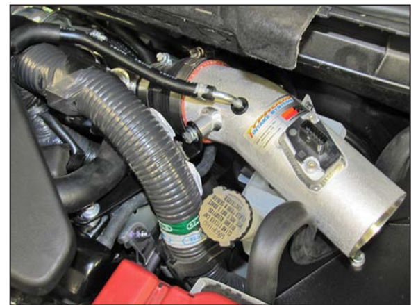
20. Insert the turbo waste gate fitting into the grommet installed into the K&N® intake tube. Use care so that the grommet is not pushed through the hole into the intake tube.
