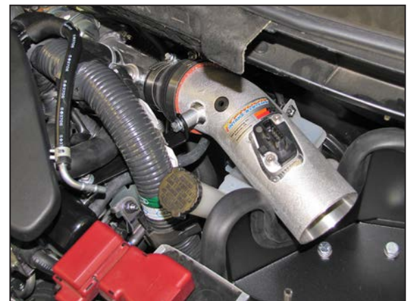
19. Install the K&N® intake tube into the coupling hose at the turbo inlet and align with the mounting bracket. Then secure the intake tube with the provided hardware and hose clamp.
