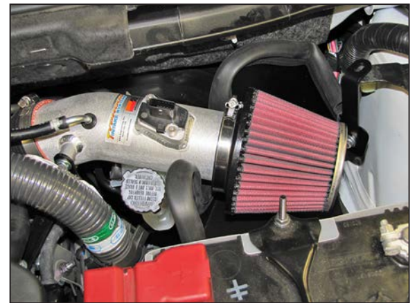
21. Install the K&N® air filter onto the intake tube and secure with the provided hose clamp.
