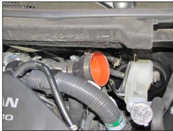
13. Install the coupling hose (5-1045) to the turbo inlet and secure with the provided hose clamp.
