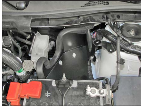
12. Install the heat shield into position on the air box mounting grommets as shown. NOTE: Do not secure the bracket at this time.
