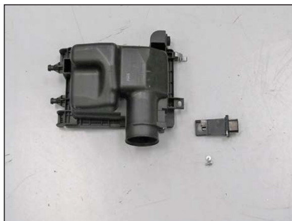
15. Remove the mass air sensor from the factory air box.
