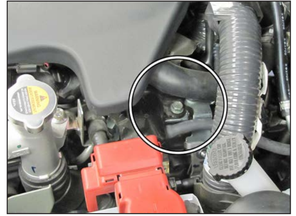
17. Remove the 6mm cover bolt shown.
