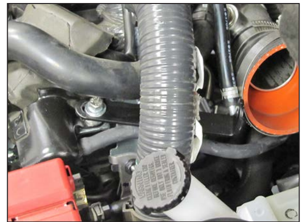
18. Install the tube mounting bracket (083164) onto the location from step #17 and secure with the provided hardware. NOTE: Be sure to place the provided spacer under the bracket.
