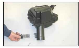
20. Remove the two screws securing the mass air sensor to the driver's side air box and then remove the mass air sensor from the air box.
