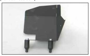
15. Install the two heat shield mounting pins onto the driver's side heat shield (074057) and secure with the provided hardware.
