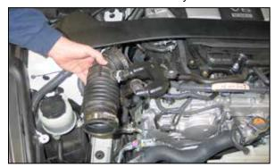
8. Remove the right side intake hose from the vehicle.
