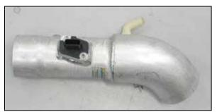
35. Install the mass air sensor into the passenger side K&N<sup>®</sup> intake tube and secure with the provided hardware.
