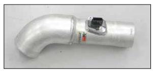
21. Install the mass air sensor into the driver's side K&N® intake tube and secure with the provided hardware.
