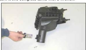
34. Remove the two screws securing the mass air sensor to the air box and then remove the mass air sensor from the air box.
