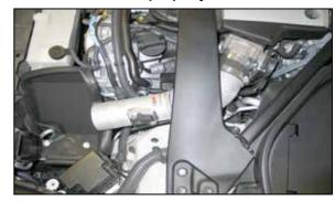
23. Install the K&N® intake tube into the silicone hose at the throttle body and align the bracket with the mounting hole in the heat shield. Adjust the tube and heat shield for proper fit and then secure with the provided hardware and hose clamp.
