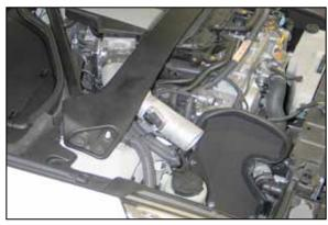
37. Install the K&N® intake tube into the silicone hose at the throttle body and align the bracket with the mounting hole in the heat shield. Adjust the tube and heat shield for proper fit and then secure with the provided hardware and hose clamp. NOTE: The tube mounting bracket is to be attached on the back side of the heat shield.
