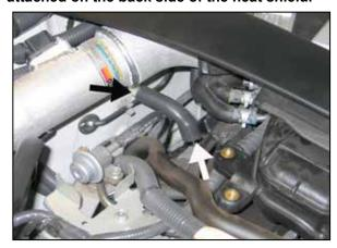
38. Install the 7" crank case vent hose onto the 90° fitting on the K&N® intake tube and then attach the open end to the vent port on the valve cover. Secure the hose to the fitting on the tube with the provided hose clamp.
