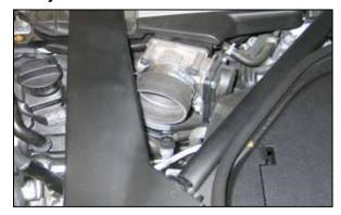
14. Install the silicone hose (084036) onto the driver's side throttle body and secure with the provided hose clamp.
