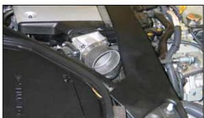
28. Install the silicone hose (084036) onto the passenger side throttle body and secure with the provided hose clamp.
