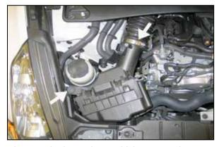
4. Loosen the hose clamp which secures the passenger side intake hose to the air box. Remove the bolt which secures the air box to the inner
