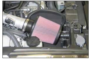
39. Install the K&N® air filter onto the K&N® intake tube and secure with the provided hose clamp.
