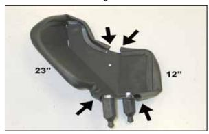
17. Install the trimmed edge trim onto the heat shield as shown.
