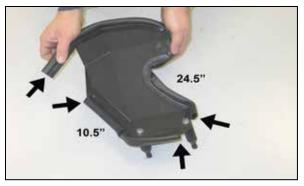
31. Install the provided edge trim onto the heat shield as shown.
