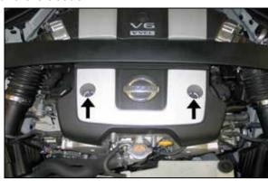
2. Remove the two bolts which secure the front engine cover and then remove the front engine cover.
