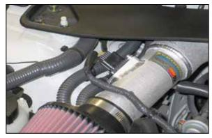
40. Reconnect the mass air sensor electrical connection.
