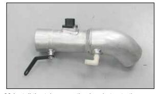
22.Install the tube mounting bracket onto the driver's side K&N® intake tube as shown and secure with the provided hardware.
