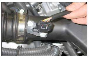
3. Disconnect the passenger side mass air sensor and unhook the wiring harness from the air box.
