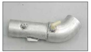
33. Install the provided 90°npt vent fitting into the  $K\&N^{\tiny \circledR}$  intake tube (27467) as shown.
