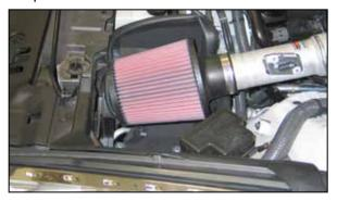
26. Install the K&N® air filter onto the K&N® intake tube and secure with the provided hose clamp. NOTE: Drycharger® air filter wrap; part # RX-4990DK is available to purchase separately.
