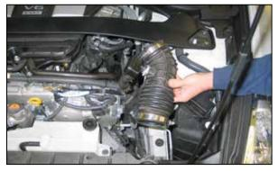
13. Remove the left side intake hose from the vehicle.
