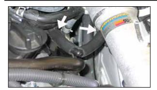
25. Connect one end of the crank case vent hose to the 90° vent fitting on the driver's side K&N® intake tube and then connect the other end to the vent port on the valve cover. Secure the hose to the fitting on the tube with the provided hose clamp.
