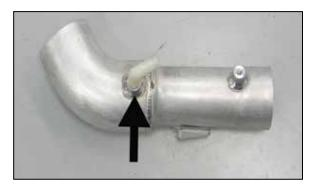
19. Install the provided 90°npt vent fitting into the driver's side K&N® intake tube (27466) as shown. NOTE: Plastic NPT fittings are easy to cross thread. Install the vent fitting "hand" tight, then turn it two complete turns with a wrench.
