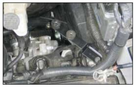
19. Install the heat shield mounting bracket assembly onto the air box mounting plate as shown and secure with the bolt from the previous step.
