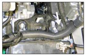
18.Remove the air box mounting plate bolt shown. **NOTE: This bolt will be reused in the next step.**
