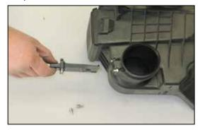
24. Remove the screws securing the mass air sensor and then remove the mass air sensor from the stock air box.
