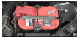
35. Reinstall the battery and secure with the factory hold down. Reconnect the positive and then the negative battery cables.
