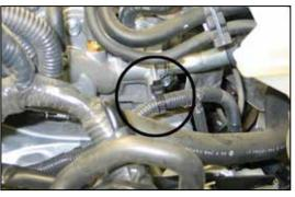
13. Unhook the wiring harness shown from the water neck housing location shown.
