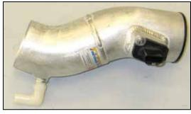
27. Install the provided 90° vent fitting onto the K&N $^{\rm @}$  intake tube as shown.
