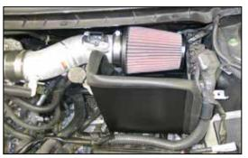
30. Install the K&N<sup>®</sup> air filter onto the intake tube and secure with the provided hose clamp. NOTE: Drycharger<sup>®</sup> air filter wrap; part # RC-9350DK is available to purchase separately.
