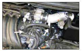
29. Install the provided silicone hose onto the crank case vent port on the valve cover and then attach the other end to the  $90^{\circ}$  fitting installed in the K&N<sup>®</sup>
