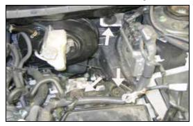
12. Remove the three air box mounting grommets shown from the air box mounts.
