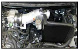
28. Install the K&N<sup>®</sup> intake tube into the silicone hose at the throttle body and align with the tube mounting bracket. Secure the intake tube with the hose clamp and hardware provided.
