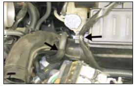
10. Disconnect the transmission vent line and wiring harness from the air box. **NOTE: The transmission vent line is held on in two locations.**
