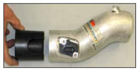
26. Install the mass air sensor venturi into the K&N<sup>®</sup> intake tube as shown. NOTE: Apply a thin coat of the provided super glue on the lip of the venturi.
