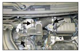
8. Loosen the two hose clamps securing the intake tube and the spring clamp securing the crank case vent hose to the valve cover.
