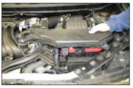
4. Lift the intake resonator up to unhook it from the three mounting grommets and then remove the resonator from the vehicle.
