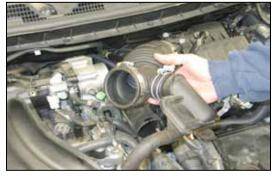
9. Remove the intake hose assembly.
