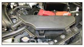
36. Reinstall the intake resonator onto the fresh air intake duct.
