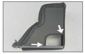
21. Install the provided edge trim into the heat shield fresh air duct opening as shown. **NOTE: Some trimming of the edge trim will be necessary.**
