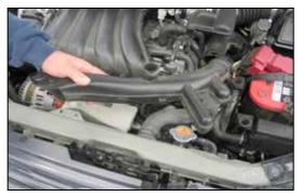
6. Remove the upper fresh air inlet duct from the vehicle.
