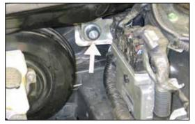
15. Install one of the provided rubber mounted studs onto the rear air box mounting bracket as shown.
