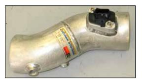
25. Install the mass air sensor into the  $K\&N^{\otimes}$  intake tube and secure with the provided hardware.
