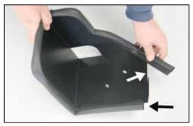
20. Install the provided edge trim onto the heat shield as shown.
