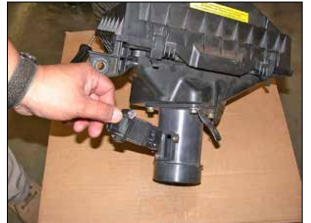
34. Remove the mass air sensor from the stock air cleaner assembly as shown.
