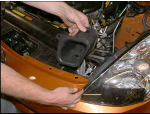
10. Pull the bumper cover forward and remove the air inlet duct as shown.
