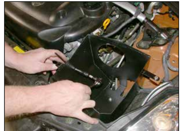
21. Adjust the air box for best fit and clearance, then tighten all the hardware on the air box as shown.
