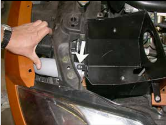
23. Secure the tube to the tab on the air box using the provided hardware but do not tighten at this time.
