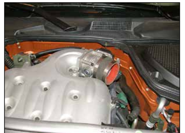
36. Install the silicone hose and hose clamps onto the throttle body as shown.
