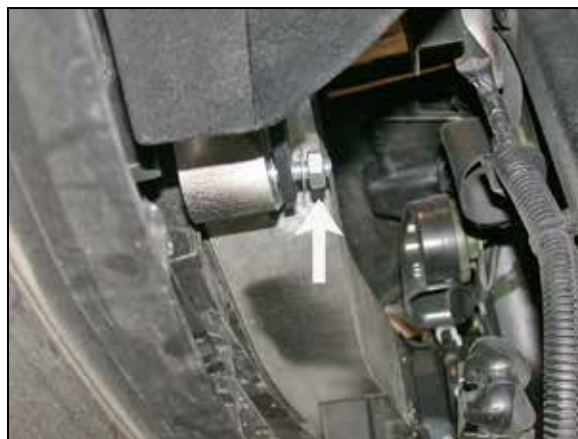
29. Slide the molded duct bracket onto the bolt from step 28, then, slide another washer and hex nut onto the hex bolt and tighten as shown.
