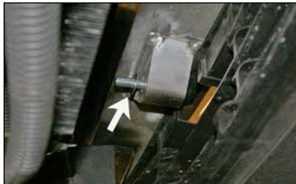
28. Slide the provided hex bolt through the aluminum cross member and slide the provided washer onto the hex bolt as shown.
