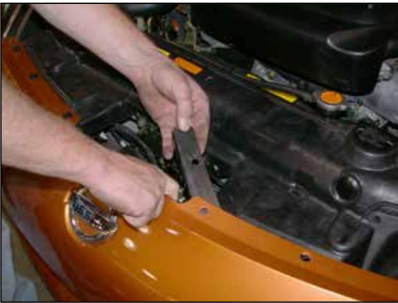
9. Loosen and remove the hex bolt that secures the Bumper cover bracket to the core support, then remove the bracket as shown.
