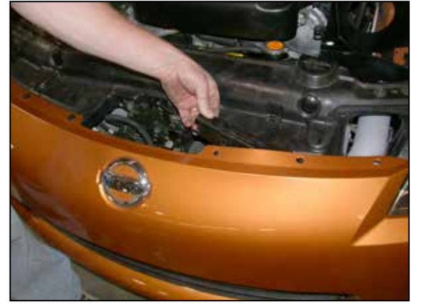
32. Reinstall the bumper cover bracket as shown and secure it with the stock hex bolt from step 9.
