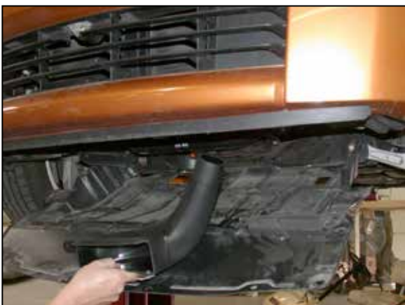
26. Install the air inlet duct from underneath the vehicle as shown.
