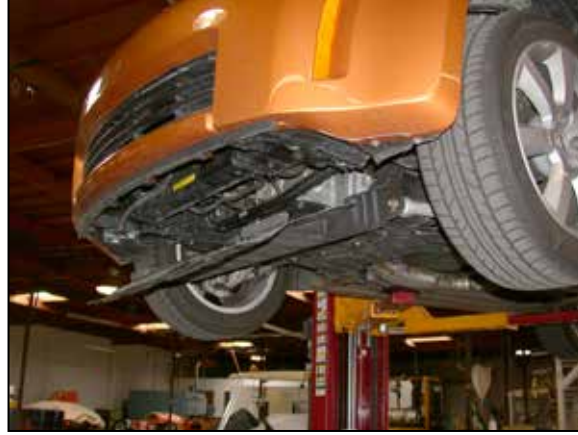
13. Remove the 12 hex bolts and 1 plastic rivet, then, lower the splash guard as shown.
