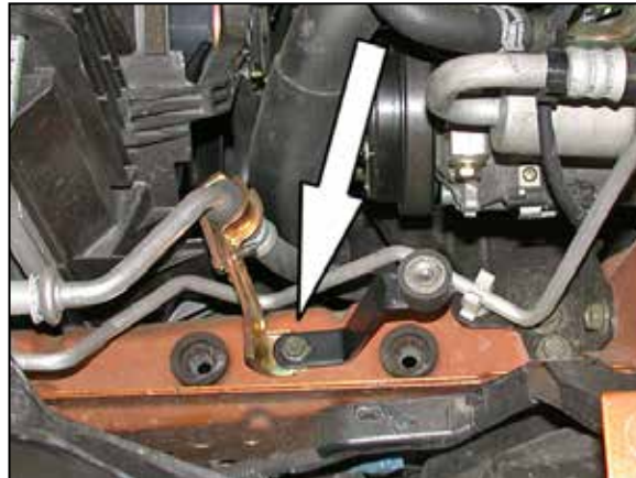
16. Using the bolt removed in step 14 secure the "Z" bracket underneath the air conditioner hardline bracket to the threaded hole from step 14. Do not tighten completely.
