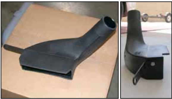
24. Install the provided bracket onto the air inlet duct using the provided hardware as shown.
