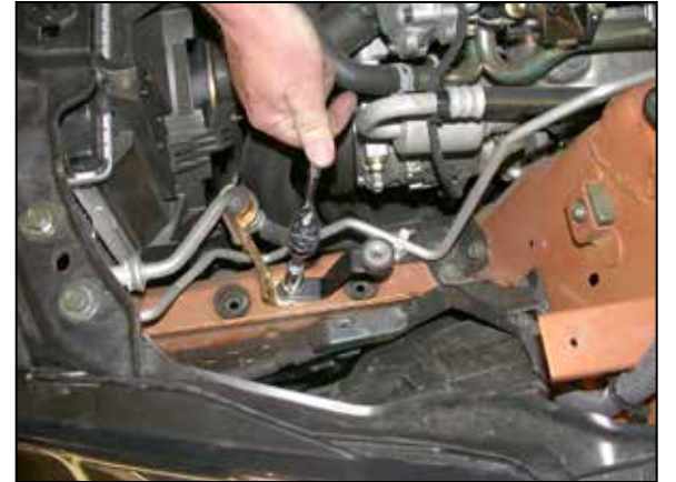
18. Remove the air box, then, tighten the "Z" bracket being careful not to move the bracket.
