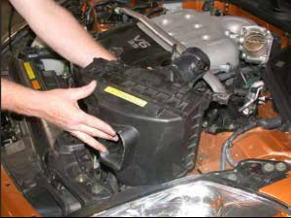
8. Pull the air cleaner assembly upwards then unclip the mass air sensor wire harness to remove the complete assembly. NOTE: K&N Engineering, Inc., recommends that customers do not discard factory air intake.
