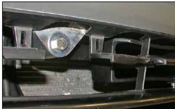
27. Slide the air inlet duct into the air inlet tube as shown, then, line up the bracket on the duct with the grille as shown.
