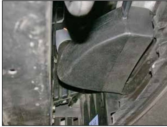
27. Slide the air inlet duct into the air inlet tube as shown, then, line up the bracket on the duct with the grille as shown.
