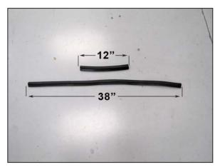
17. Cut the provided edge trim into two sections. One section should be cut to 12" long and the next section should be cut to 38" long.
