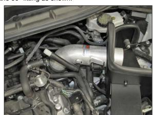
25. Pass the intake tube through the heat shield and then install it into the hose at the throttle body. Then secure the tube with the provided hose clamp.
