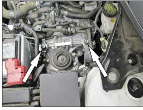
12. Mount the two rubber mounted studs to the air box mounting brackets as shown.
