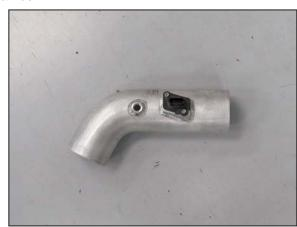
21. Install the mass air sensor into the K&N® intake tube and secure with the provided hardware.
