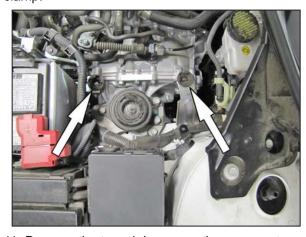
11. Remove the two air box mounting grommets from the mounting brackets shown.
