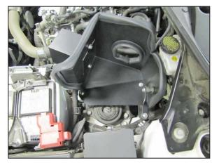
19. Install the heat shield assembly onto the rubber mounted studs and secure with the provided hardware.
