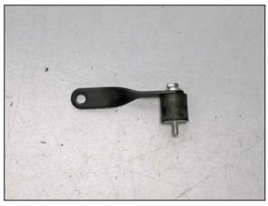
15. Install the remaining  $\frac{1}{2}$ " long stud onto the upper air box mounting bracket as shown.
