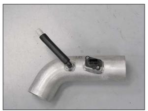
24. Install the crank case vent hose assembly onto the 90° fitting as shown.
