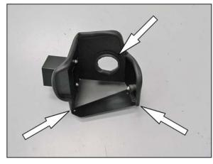
18. Install the 12"long section into the hole of the heat shield and install the 38"long section around the outside of the heat shield.
