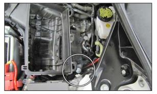
6. Remove the bolt which secures the lower air box to the mounting bracket. Remove the lower air box from the vehicle.
