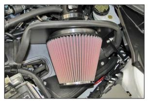
23. Install the K&N<sup>®</sup> air filter onto the filter adapter and secure with the provided hose clamp. **NOTE: Drycharger<sup>®</sup> air filter wrap; part # RF-1048DK is available to purchase separately.**
