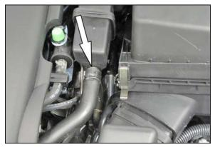
4. Release the spring clamp securing the crank case vent hose to the intake plenum and then disconnect the crank case vent hose.
