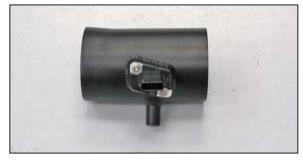
18. Install the mass air sensor into the  $K\&N^{\circledast}$  intake tube and secure with the provided hose clamp.
