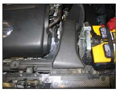
21. Reinstall the intake duct onto the core support and into the heat shield assembly. Secure with the factory bolts.
