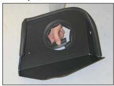
15. Install the provided edge trim into the hole of the heat shield as shown.
