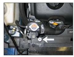
2. Remove the bolt that secures the fresh air intake scoop shown. This bolt will be reused.
