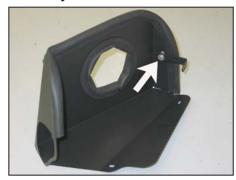
17. On manual transmission equipped vehicles, install heat shield mounting bracket #07195 onto the heat shield as shown. On automatic transmission equipped vehicles, install heat shield mounting bracket #010040.
