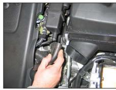
6. Release the crankcase vent hose spring clamp and then disconnect the crankcase vent hose from the intake tube resonator chamber.
