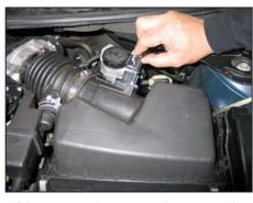
7. Disconnect the mass air sensor electrical connection.
