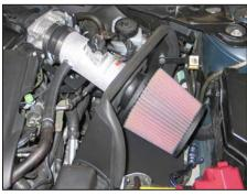
29. Install the K&N® air filter onto the intake tube and secure with the provided hose clamp.
