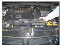
5. Remove the fresh air intake duct from the vehicle as shown.
