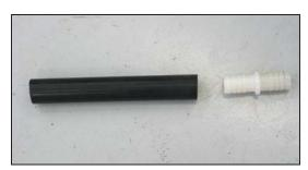
27. Install the hose mender into the crankcase vent hose provided.
