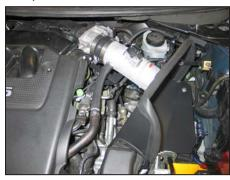
28. Install the crankcase vent hose into the factory crankcase vent hose and then connect the open end onto the  $K\&N^{\otimes}$  intake tube as shown.
