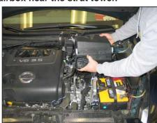
9. Loosen the hose clamp, which secures the intake tube to the throttle body. Remove the complete stock intake assembly from the vehicle. NOTE: K&N Engineering, Inc., recommends that customers do not discard factory air intake.
