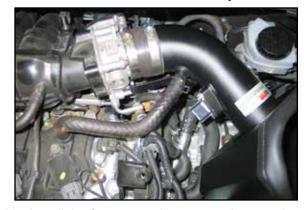
23. Install the factory crank case vent hose to the  $1\!\!/\!_{\!\!4}\!^{n}$  npt vent installed onto the K&N® intake tube.
