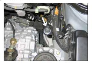
11. Install the  $\frac{1}{2}$ " high rubber mounted stud onto the rear air box mounting location using the provided hardware.
