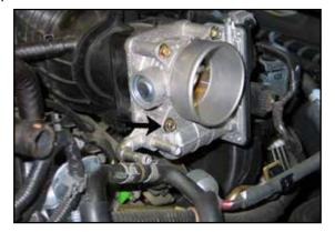
12. Remove the lower-front throttle body mounting bolt.
