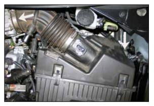
7. Loosen the hose clamp which secures the intake hose to the throttle body and remove the air box mounting bolt.
