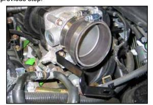
14. Install the provided silicone hose (084036) onto the throttle body and secure with the provided hose clamp.
