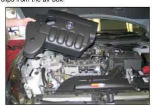
3. Remove three bolts which secure the engine cover and then remove the engine cover.
