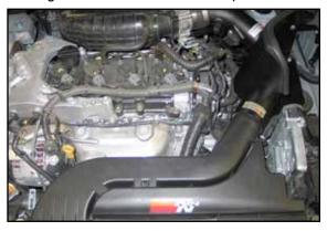
22. Reinstall the fresh air inlet supply to the original location and into the fresh air tube on the heat shield then secure with the factory bolts.
