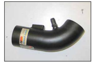
15. Install the provided 1/4"npt vent fitting into the K&N® Intake Tube as shown.
