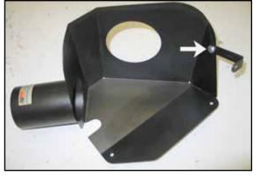
19. Install the heat shield mounting bracket (010051) onto the heat shield as shown using the provided hardware.
