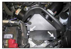
21. Install the heat shield into the vehicle so the mounting holes line up with the rubber mounted studs installed earlier. Secure the heat shield and mounting bracket with the hardware provided.
