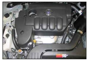
26. Reinstall the engine cover and secure with the factory bolts.
