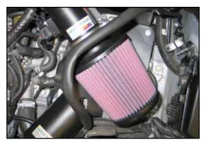
25. Install the K&N® air filter onto the K&N® intake tube and secure with the provided hose clamp. NOTE: Drycharger® air filter wrap; part # RU-4990DK is available to purchase separately.
